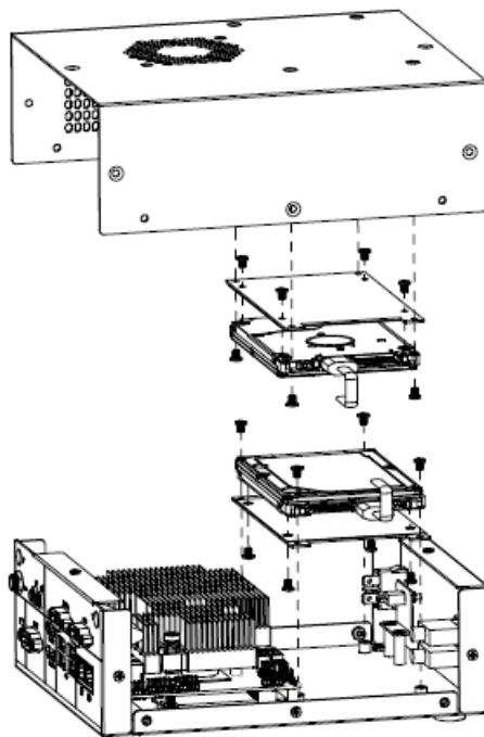
**Step1.** For SSD installation, please remove the top cover, Fix SSD using the 8 screws in the Accessory Kit.
