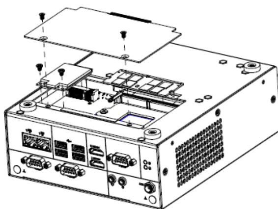
**Step2.** For Memory and Mini PCIe installation, Unfasten 2 screws to remove the cover.
