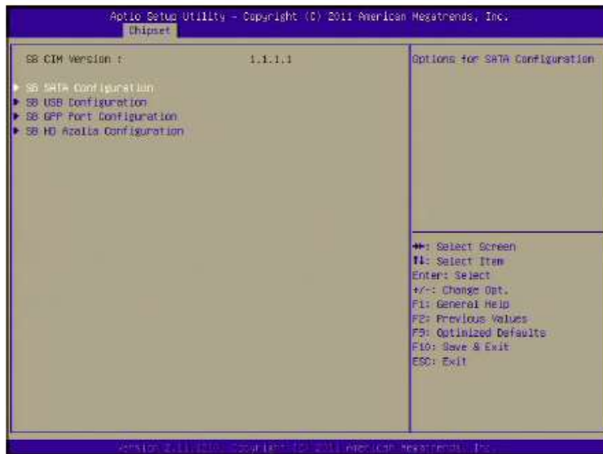
Figure 3.16 South Bridge Setup Screen
