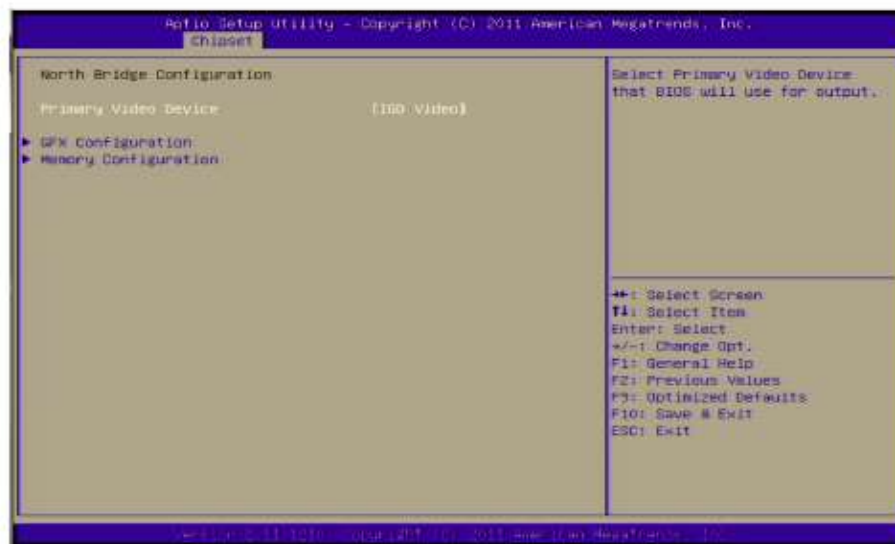
Figure 3.12 North Bridge Configuration Screen
