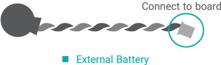
The external lithium ion battery supplies power to the real-time clock and CMOS memory as an auxiliary source of power when the main power is shut off.
