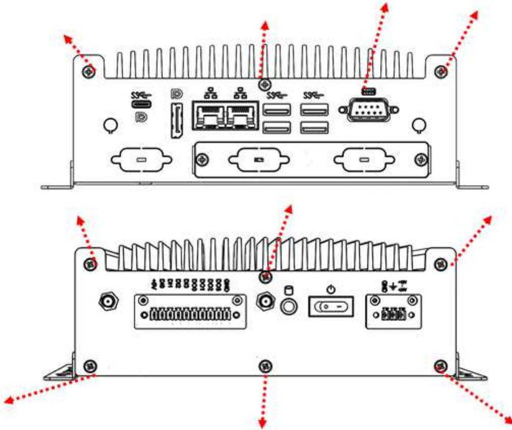
2. Remove the 2 screws shown below and proceed to install the M.2 card.
