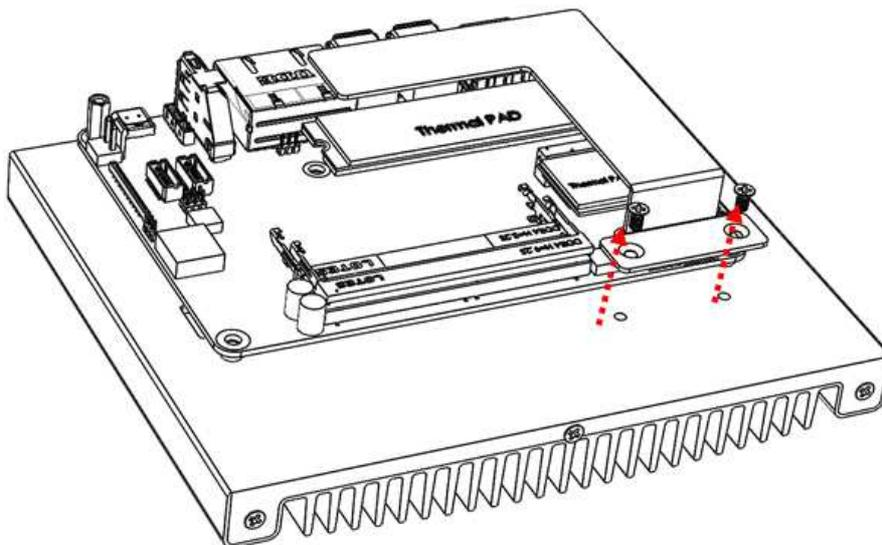
3. Align the key of the m.2 card to the m.2 interface, and insert the card slantwise.
