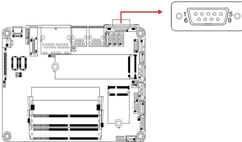
COM1 port is jumper-less and configurable in BIOS.
