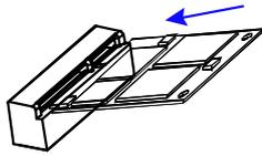
4. Push the m.2 card down, fix it onto the standoff with a screw.
