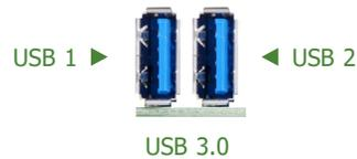
USB allows data exchange between your computer and a wide range of simultaneously accessible external Plug and Play peripherals. The PIC-Q170/H110 is equipped with two onboard USB 3.0 ports (USB 1&2) at the rear side.
