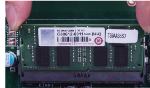
6. Push down the module until the clips at each end of the socket lock into position. You will hear a distinctive "click", indicating the module is correctly locked into position.
