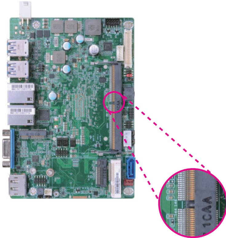
5. Grasping the module by its edges, align the module into the socket at an approximately 30 degrees angle. Apply firm even pressure to each end of the module until it slips down into the socket. The contact fingers on the edge of the module will almost completely disappear inside the socket.
