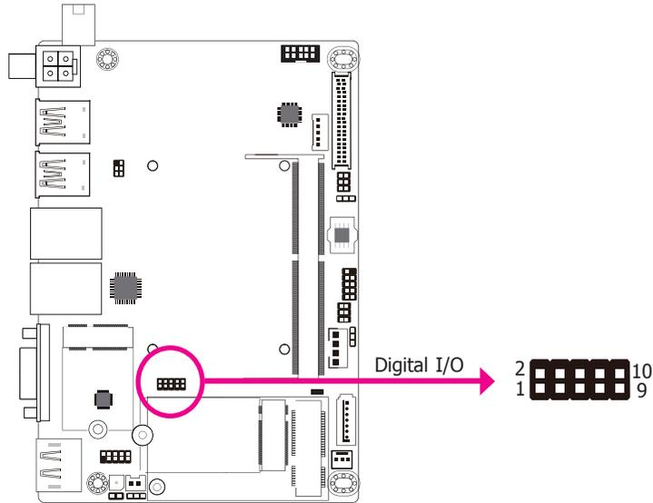
The 8-bit Digital I/O connector provides monitoring and control functions to the connected external devices.
