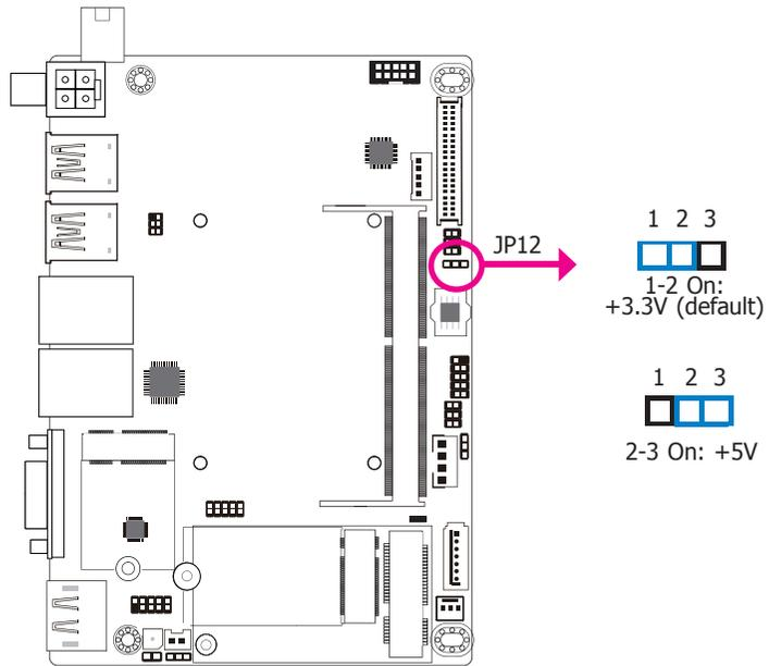
JP12 is used to select the power level of backlight brightness control: +3.3V or +5V.
