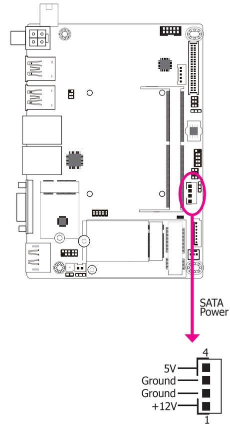
The SATA power connector supplies power to the SATA drive. Connect one end of the provided power cable to the SATA power connector and the other end to your storage device.
