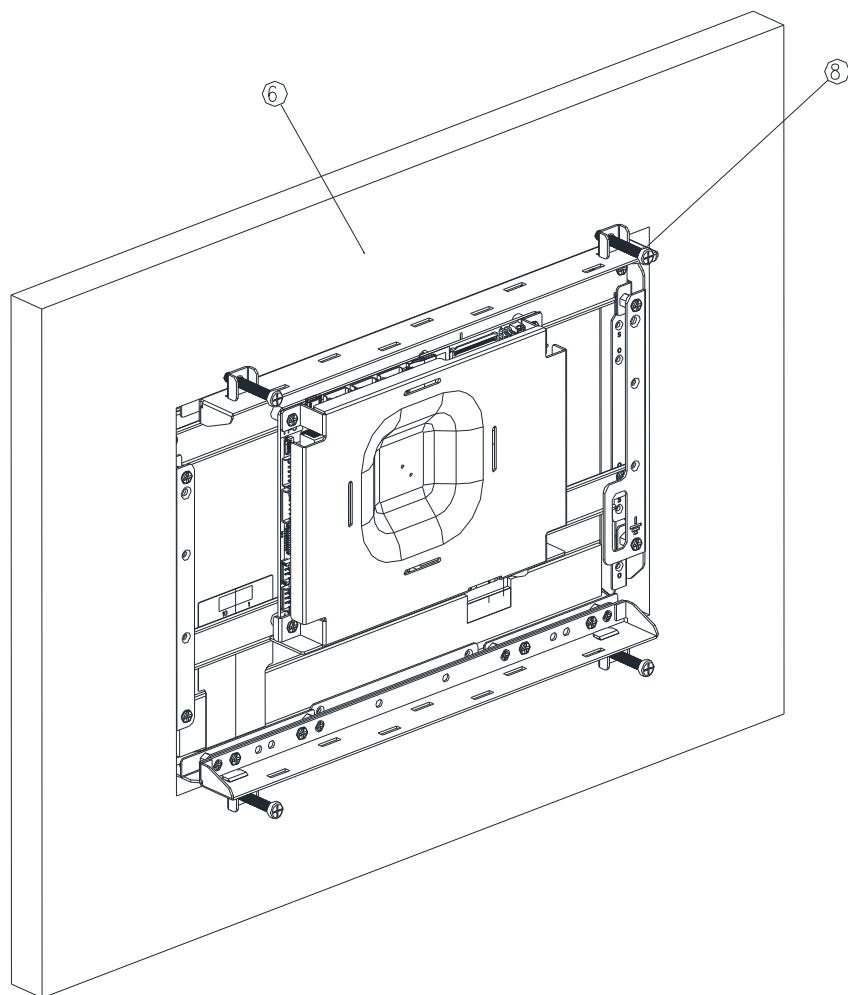
**Step6.** Insert and fasten 4 Panel mount screws to secure the module.
