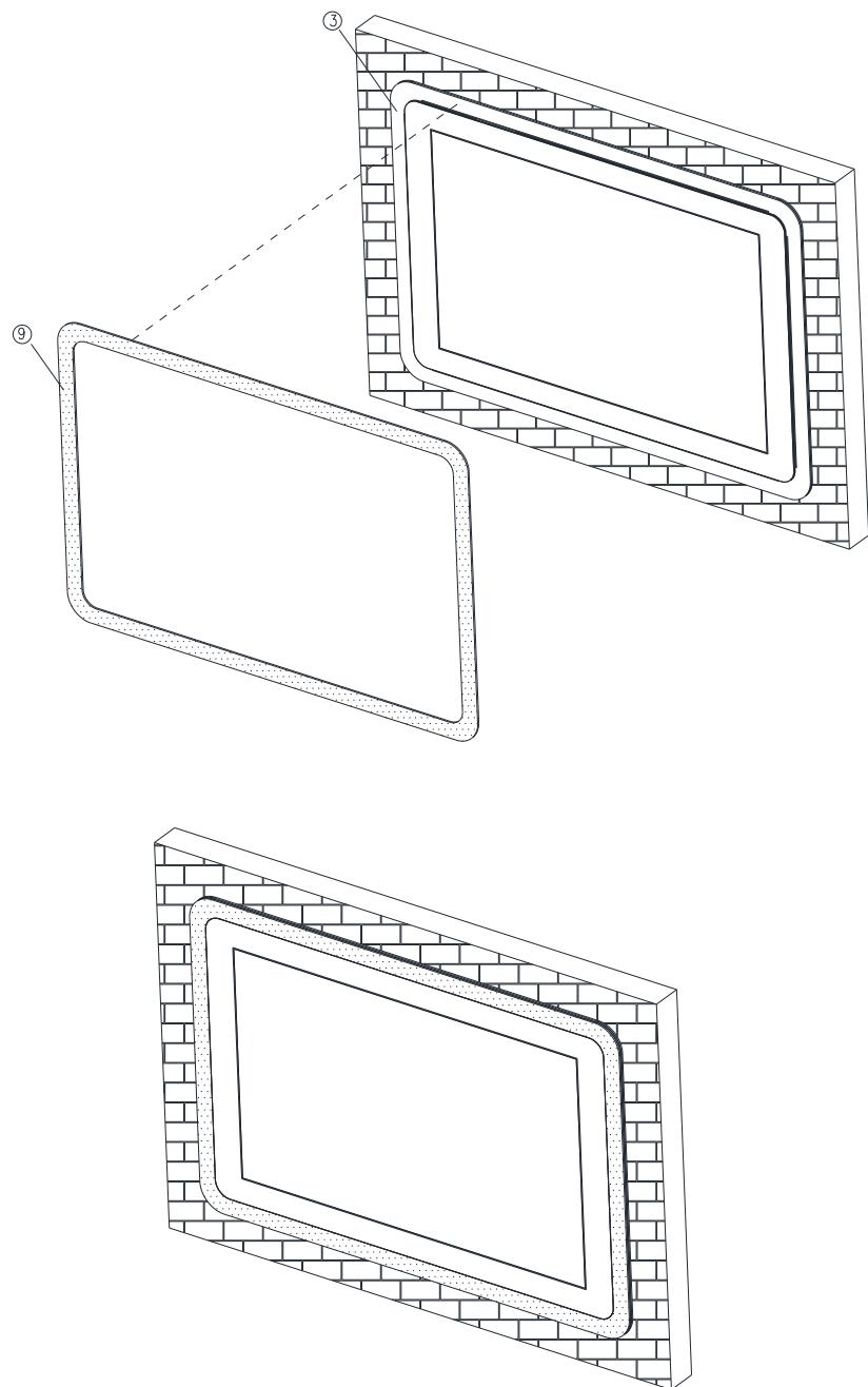
**Step7.** Paste the Decoration Plate on the Front bracket to complete installation.
