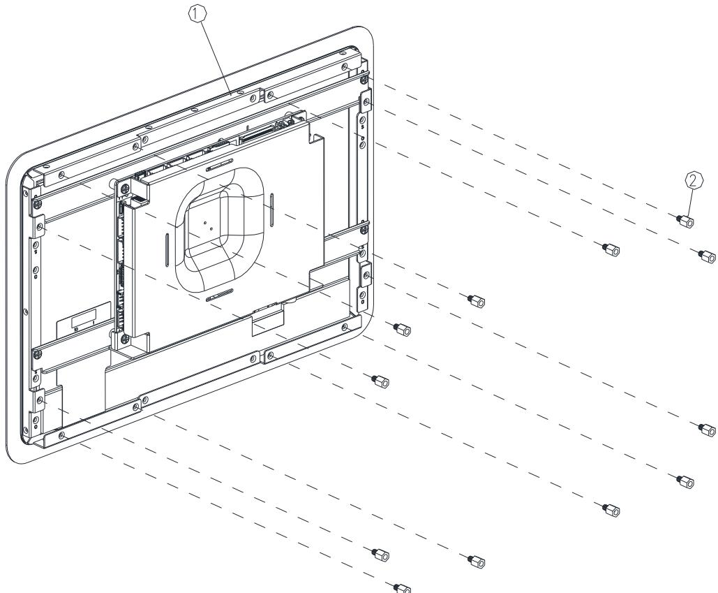
**Step1-1.** Locate brackets on both sides, matching the holes on the monitor.
