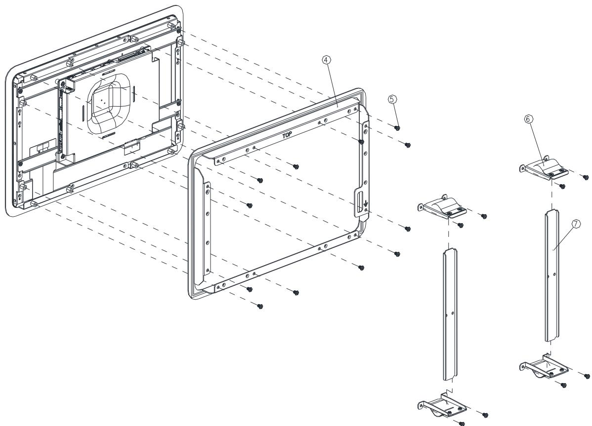
**Step3-1.** Insert and fasten 12 screws on each side of the monitor to secure Front bracket.
