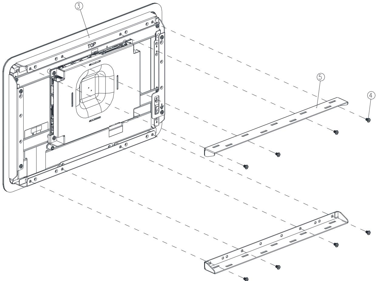
**Step3.** Insert and fasten 8 screws to secure Bracket T/B.
