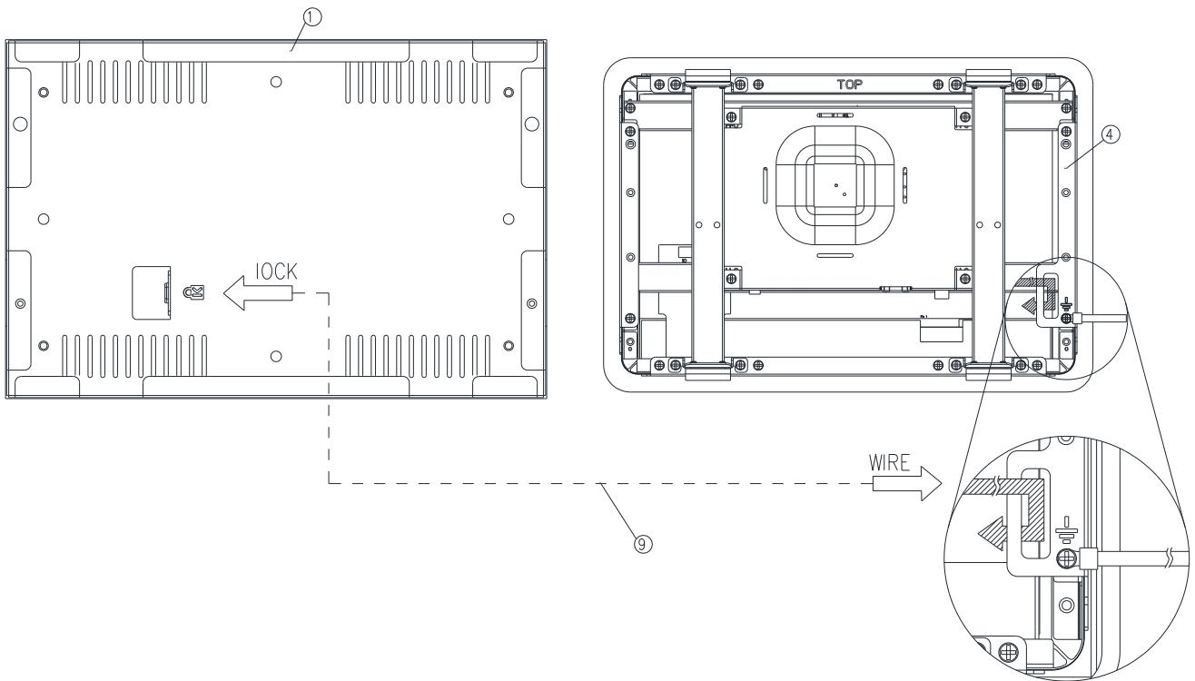
**Step5.** Wrap the Kensington lock (option) around the hole in the front bracket and attach the lock to the keyhole in the Wall box.
