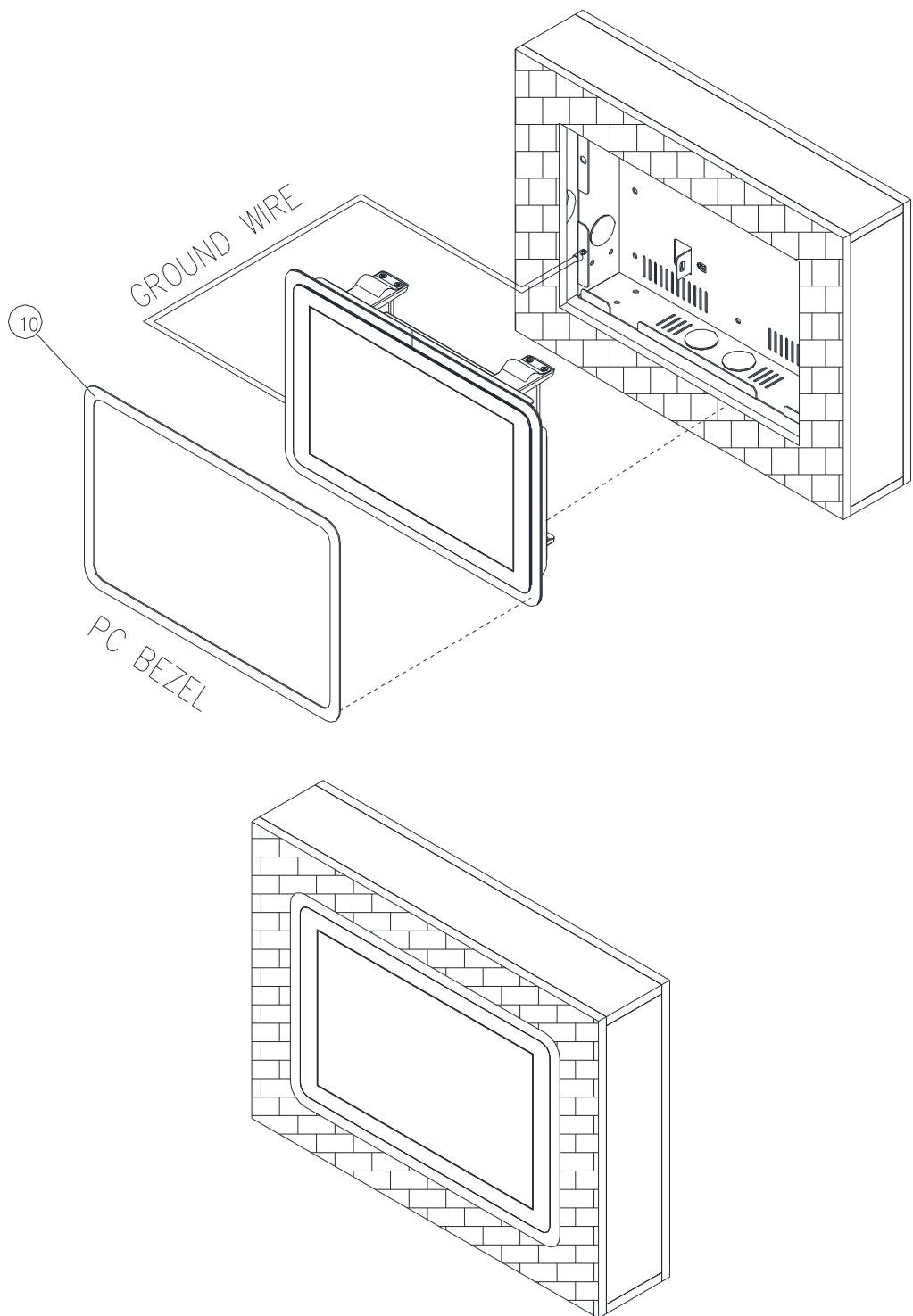
**Step6-1.** Insert the Ground wire and Kensington lock in the Wall box and Insert OFT-10WR1 into the wall.
