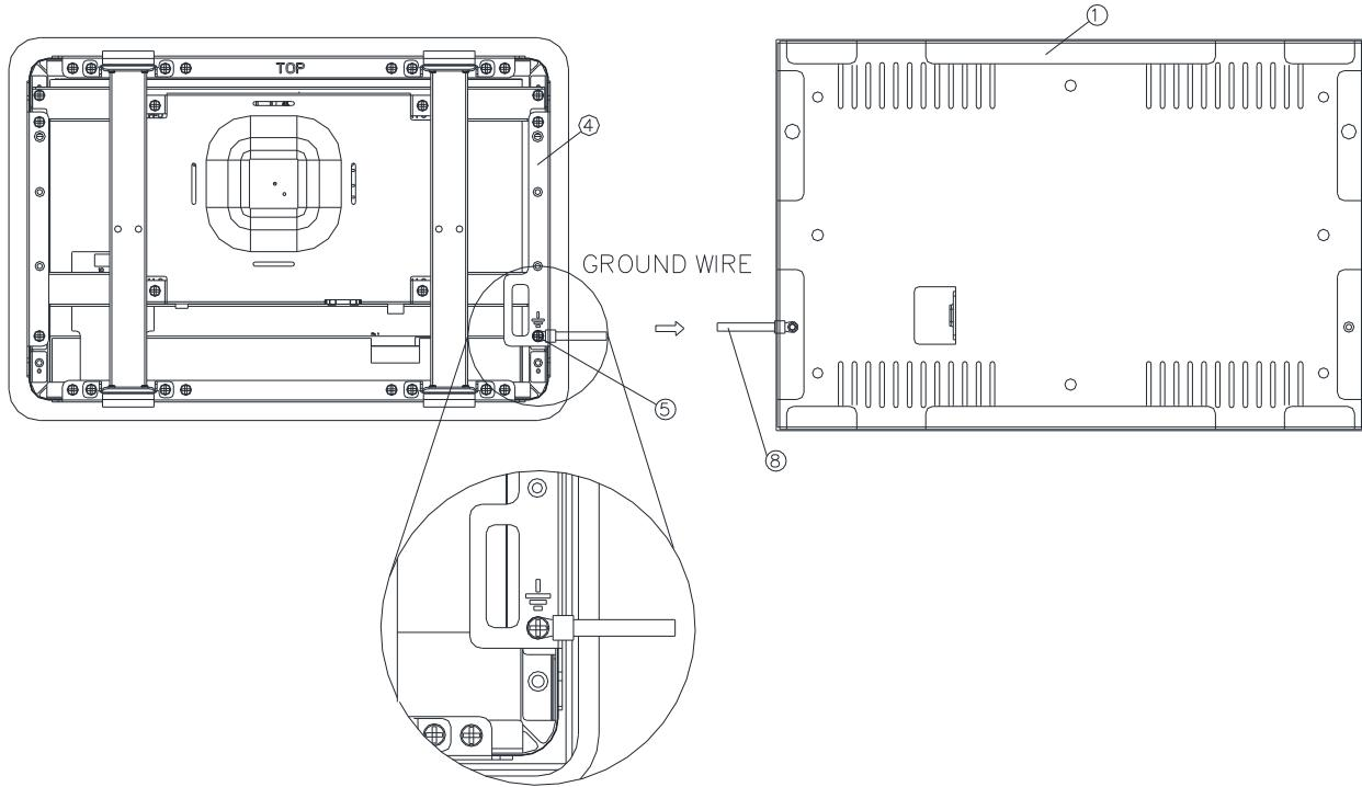
**Step4.** Insert and fasten 2 screws on Front bracket and Wall box of the monitor to secure Ground wire.
