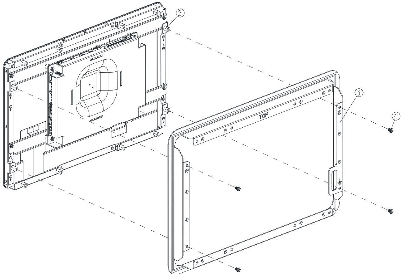
**Step2.** Insert and fasten 4 screws on each side of the monitor to secure Front bracket.
