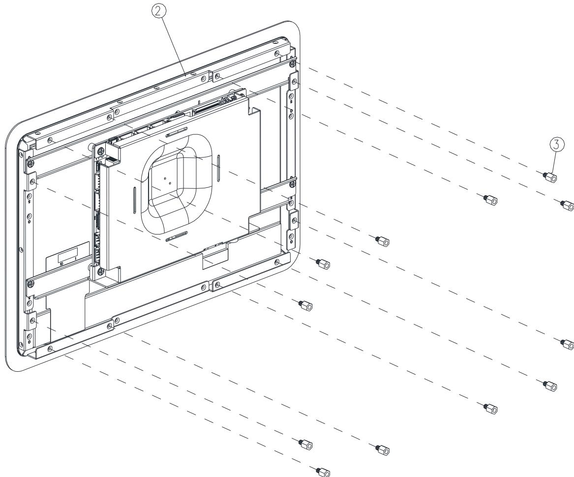
**Step2.** Insert and fasten 12 screws on each side of the monitor to secure brackets.
