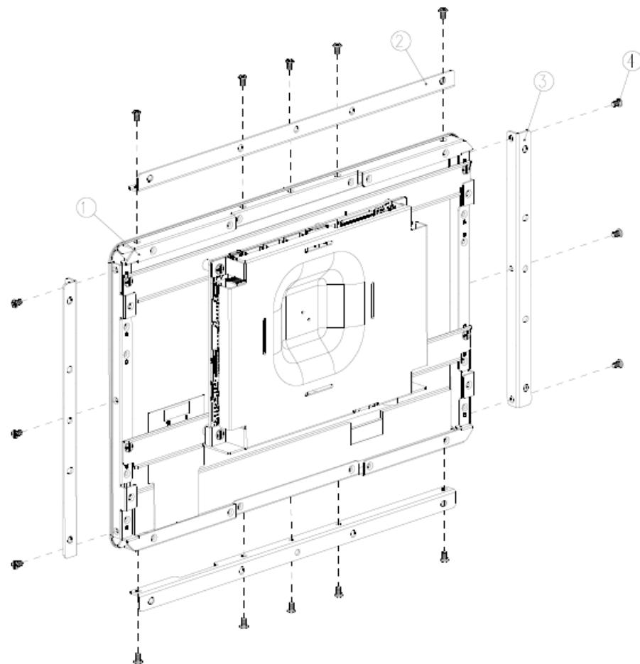
**Step1.** Locate brackets on both sides, matching the holes on the monitor.
