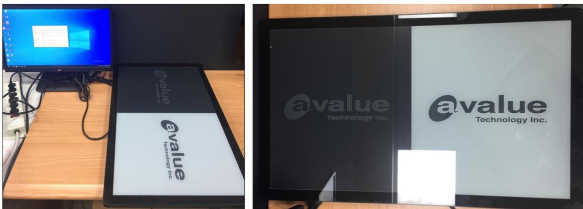
g. Check “Single” and then choose the folder’s picture you want to show constantly. The picture needs to comply with the EPD resolution. For example, EPD-3133’s resolution is 2560 x 1440, so the picture needs to be 2560 x 1440 resolution. The picture format needs to be BMP.
