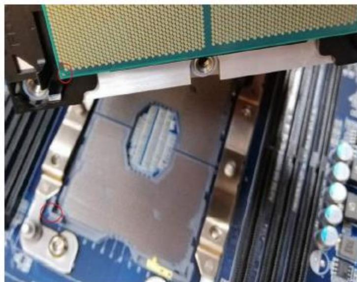
**Step7.** Please keep Pin1 as red-circled aligned with CPU when installing.
