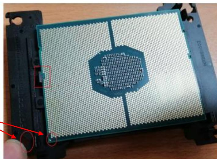
**Step4.** To turn upside down of the Blaster and install CPU on this side. To notice the red circle marking of the Pin1, and the red square marking of the latch.
