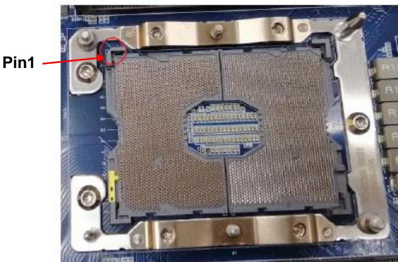
**Step2.** To be careful of the diagonal location on the socket of Pin1 as above photo on red circle marking.
