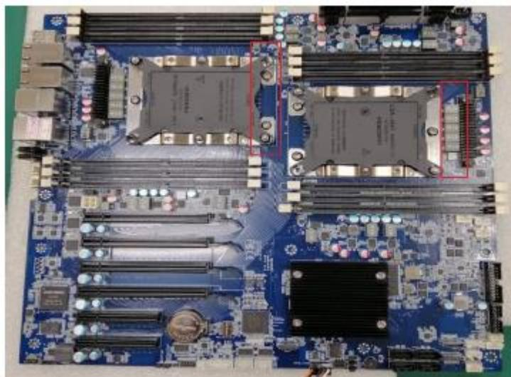
To notice the orientation of the FAN as the red square marking of photo when installing the CPU heatsink module to the motherboard.
