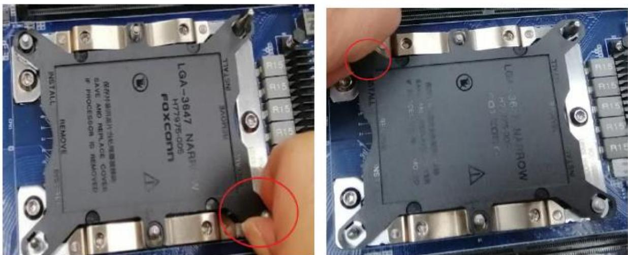
**Step1.** To remove CPU socket cover and be careful of the latch on diagonal location as the red circle marking above photo.
