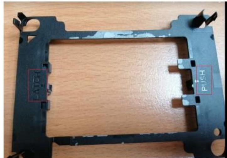
**Step3.** There is marking of PUSH and LATCH on the Blaster. Heatsink cooler need to be installed on this side.
