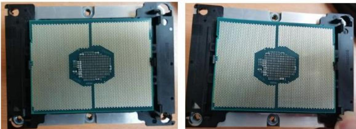
**Step6.** To install 4 corners of CPU and Blaster to the heatsink.
