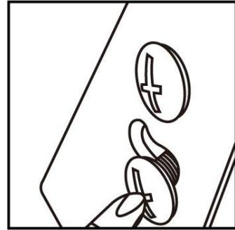
3. Secure tightly locking handle to the Panel PC.
