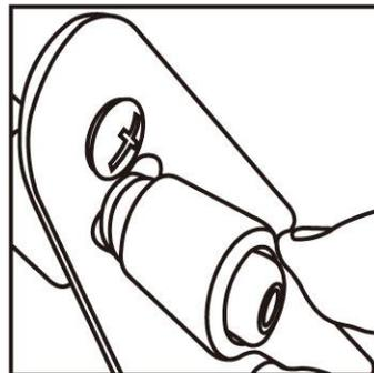
4. Loosen the hand-screw adjustment tool, then you can adjust product angle on the stand. Then screw the product tightly again to secure the stand position.
