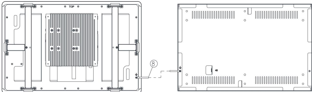
**Step3.** Fasten the Ground wire with 2 screws on the ground screw holes of OFT-15W04 and Wall box.
