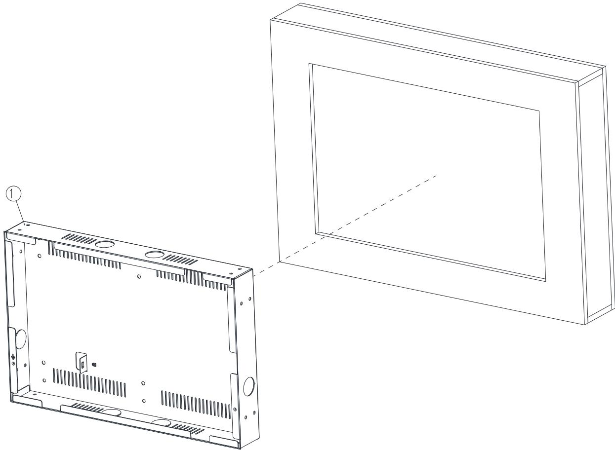
**Step1.** Install the 15" Wall Box and fix it on the wall, and use suitable screws to lock the wall box (the screws can be purchased according to actual needs).
