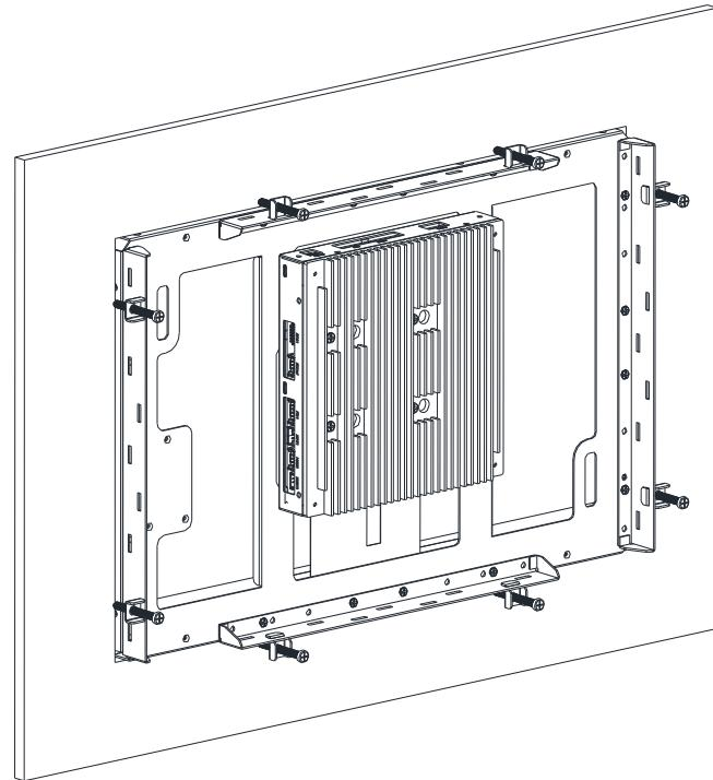
**Step4.** Insert and fasten 8 Panel mount screws to secure the module.
