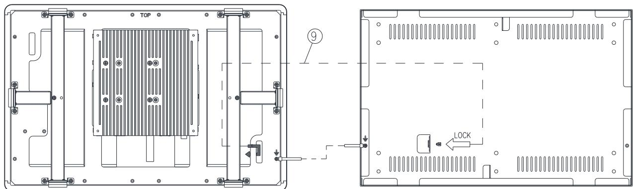
**Step4.** Wrap the Kensington lock (option) around the hole in the OFT-15W04 and attach the lock to the keyhole in the Wall box.
