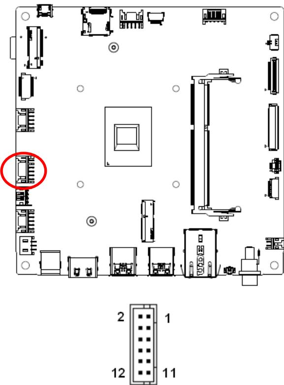
**Note:** When using cable to connect JTB1 connector, please use twisted cable.
