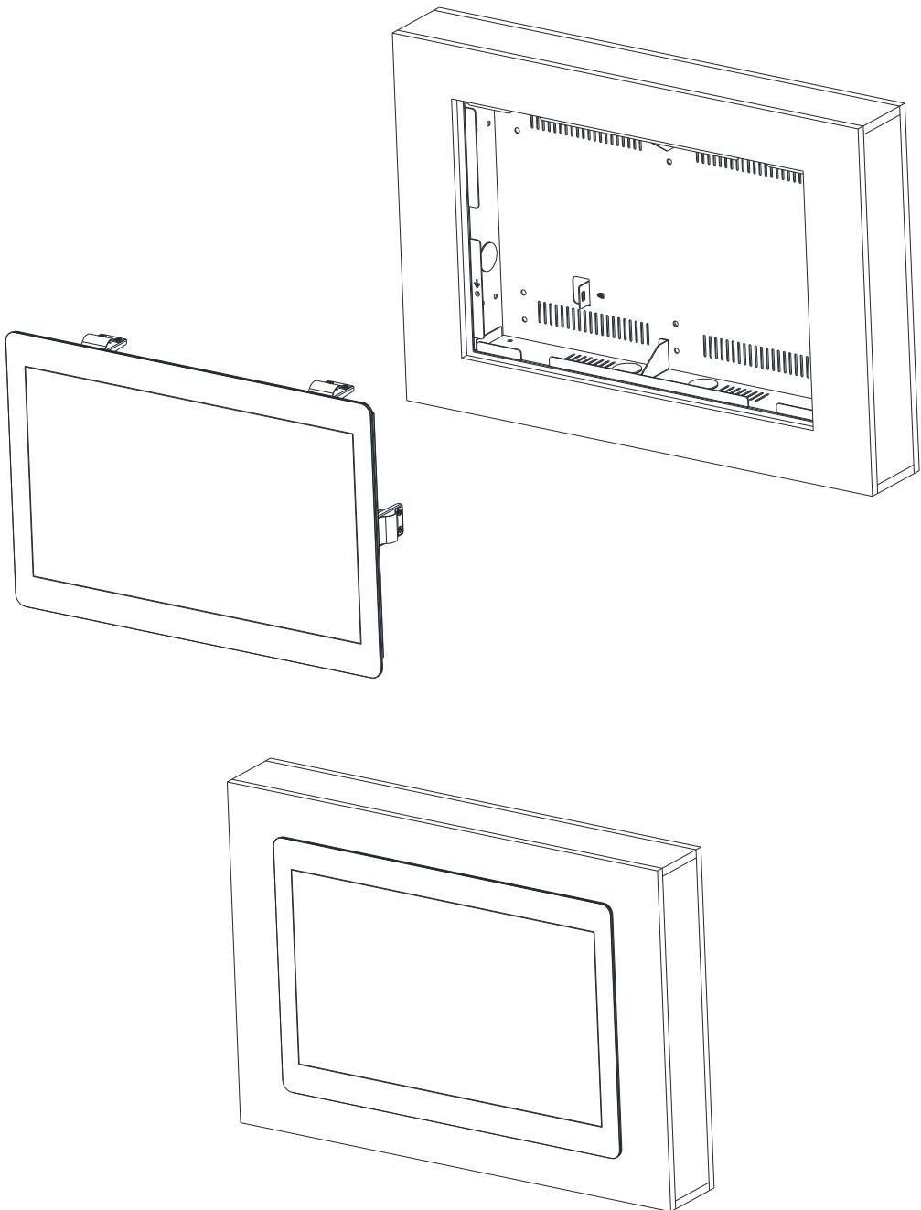
**Step5.** Store the Ground wire and Kensington lock in the Wall box and embed the OFT-15W04 into the wall (Wall Box).
