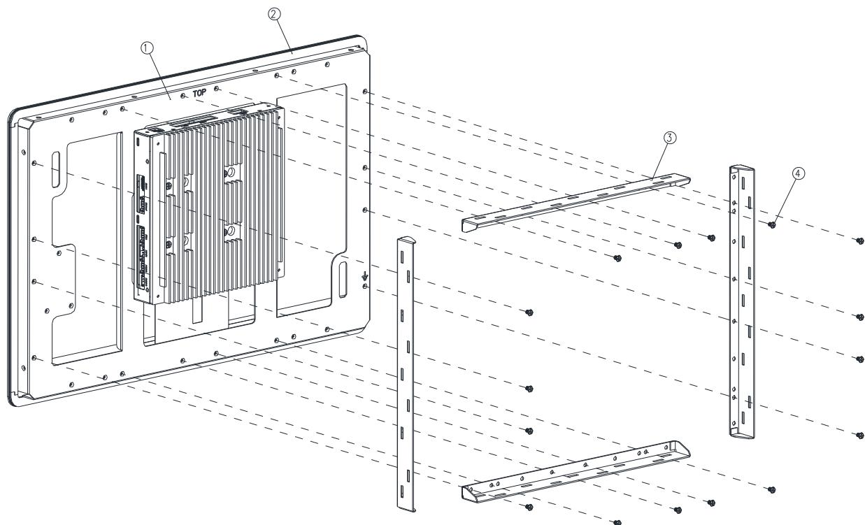
**Step1.** Insert and fasten 16 screws to secure Panel mount brackets.
