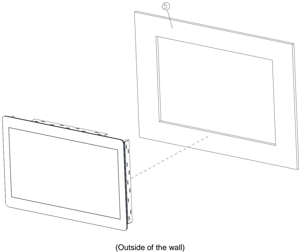
**Step2.** Insert OFT-15W04 Open frame into the wall.
