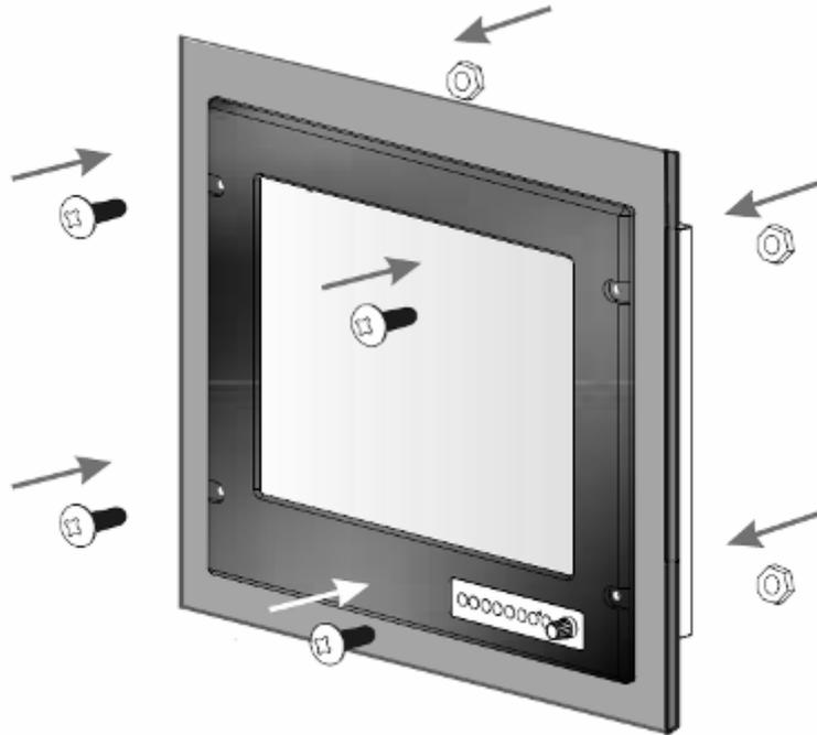
**Step2.** Use M4x 15mm bolts to drill through the fixture into the mounting holes on the rear side of IP65 front bezel.(The quantity of mounting screws based on drawing)
