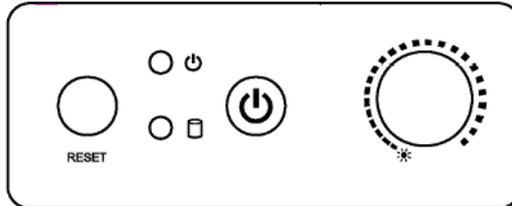
Figure 3.2 In Front User Controls ( for 10.4 inch to 17inch)
