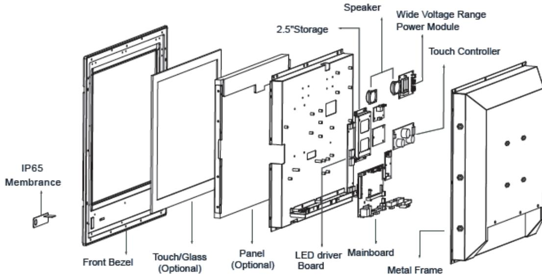
Figure 1.1 Basic Construction
