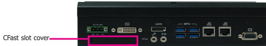
2. Gently insert the CFAST card straight with the label on the CFAST card facing up until you feel it lock into place. Do not force the card into the slot if the card is not correctly inserted.
