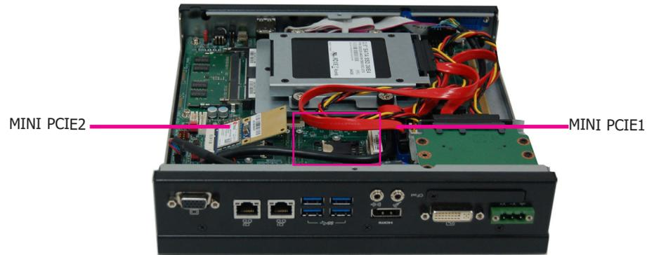
2. Push the Mini PCIe card down and use the provided mounting screws to secure the card on the system board.
