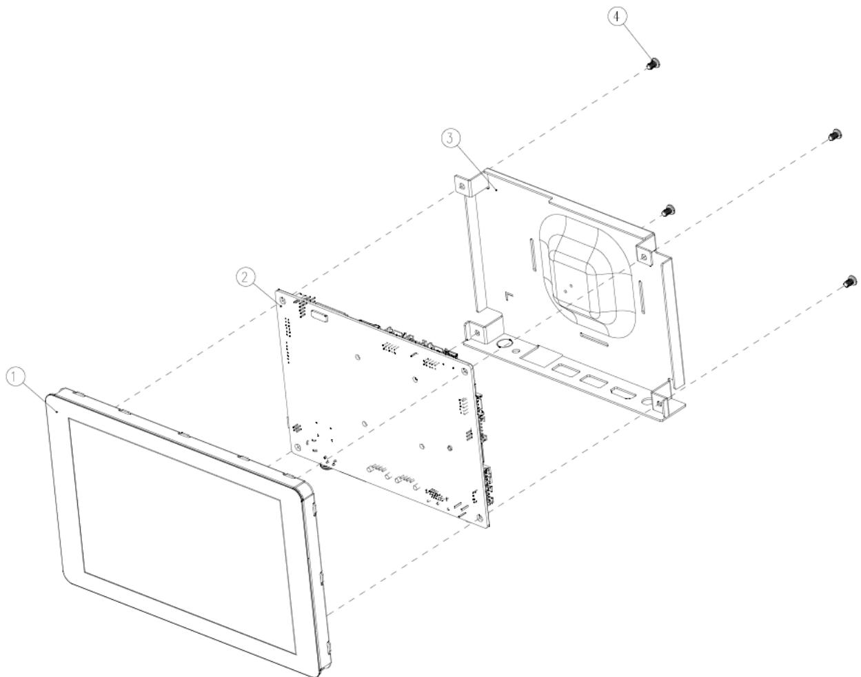
**Step1.** Locate brackets on both sides, matching the holes on the monitor.
