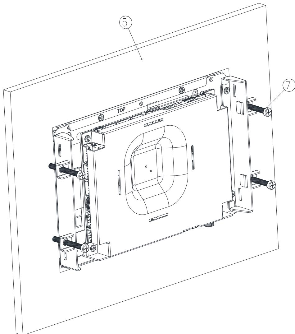
**Step6.** Insert and fasten 4 Panel mount screws to secure the module.
