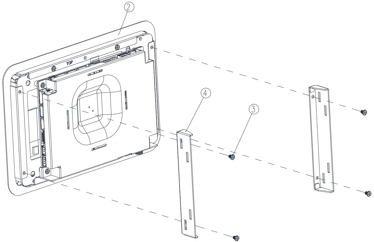
**Step3.** Insert and fasten 4 screws to secure Bracket R/L.
