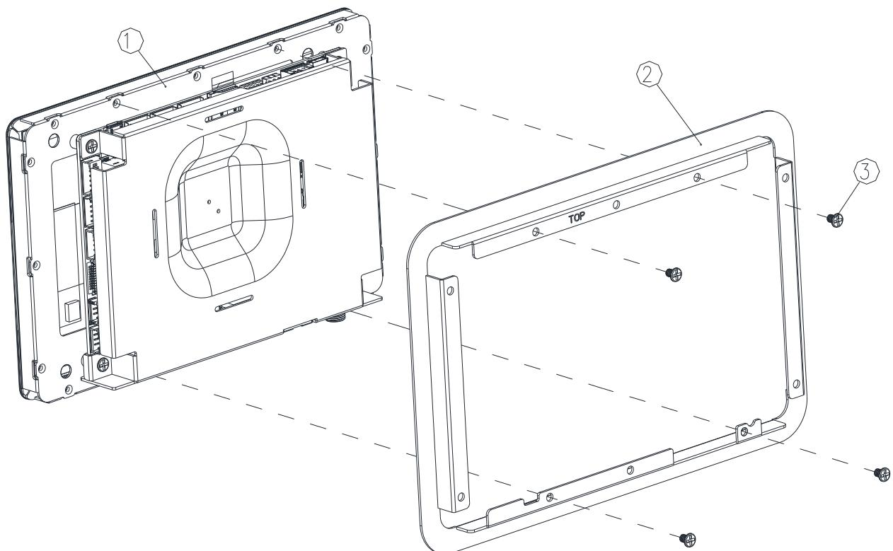
**Step2.** Insert and fasten 4 screws on each side of the monitor to secure Front bracket.
