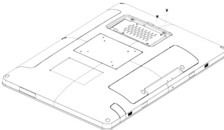
Insert the HDD back and fasten 2 screws.
