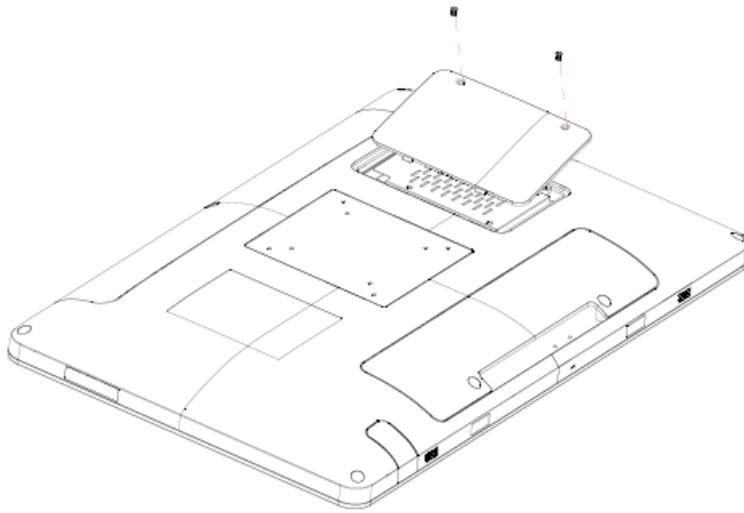
Remove 2 screws to release the chassis cover, and remove it.
