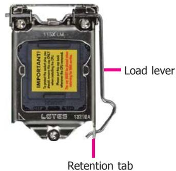
5. Lifting the load lever will at the same time lift the load plate.
