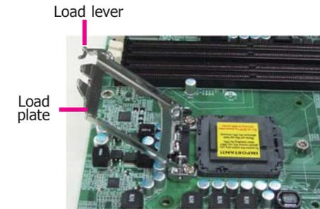
6. Remove the protective cap from the CPU socket. The cap is used to protect the CPU socket against dust and harmful particles. Remove the protective cap only when you are about to install the CPU.
