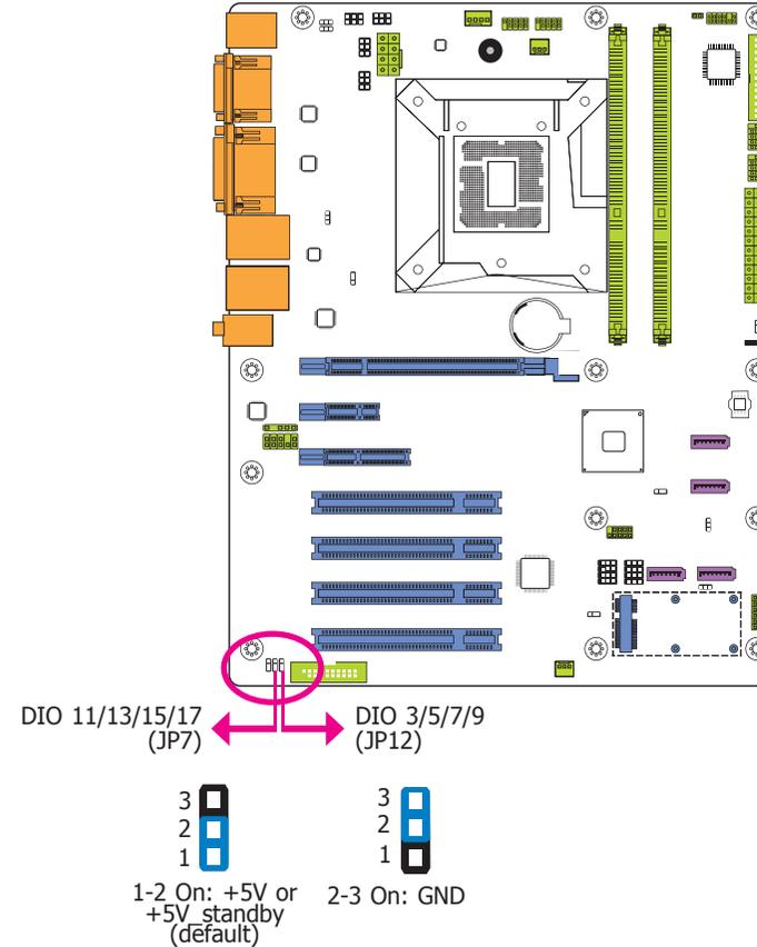
Based on the power level of DIO (Digital I/O) selected on JP13, JP12 (DIO pin 3/5/7/9) and JP7 (DIO pin 11/13/15/17) are used to select the state of DIO output: pull high or pull low. When selecting pull high, the power selection will be the same as JP13's setting.
