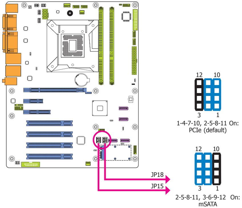
JP15 and JP18 are used to select the Mini PCIe signal.
