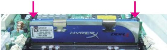
8. The ejector tabs at the ends of the socket will automatically snap into the locked position to hold the module in place.
