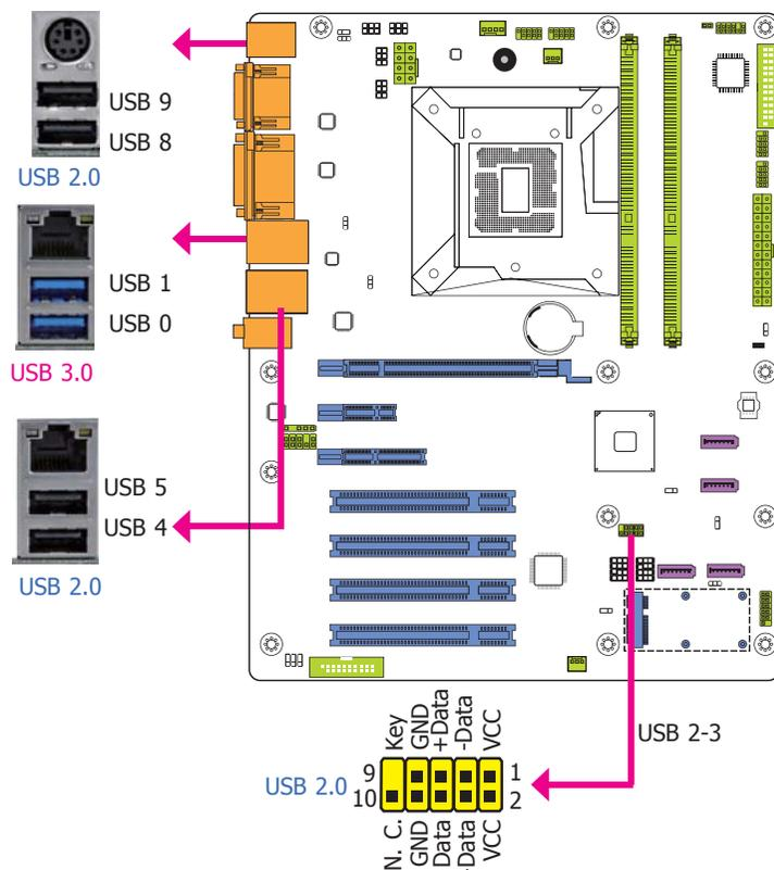
The USB device allows data exchange between your computer and a wide range of simultaneously accessible external Plug and Play peripherals.
