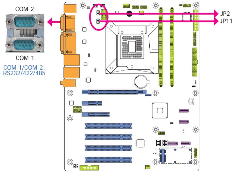
JP2 (for COM1) and JP11 (for COM2) are used to configure the COM ports to RS232, RS422 (Full Duplex) or RS485. The pin functions of the COM ports will vary according to the jumper's setting.
