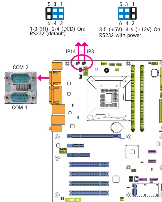
JP3 (for COM 1) and JP14 (for COM 2) are used to configure Serial COM ports to pure RS232 or RS232 with power. The pin functions of COM 1 and COM 2 will vary according to JP3's and JP14's setting respectively.
