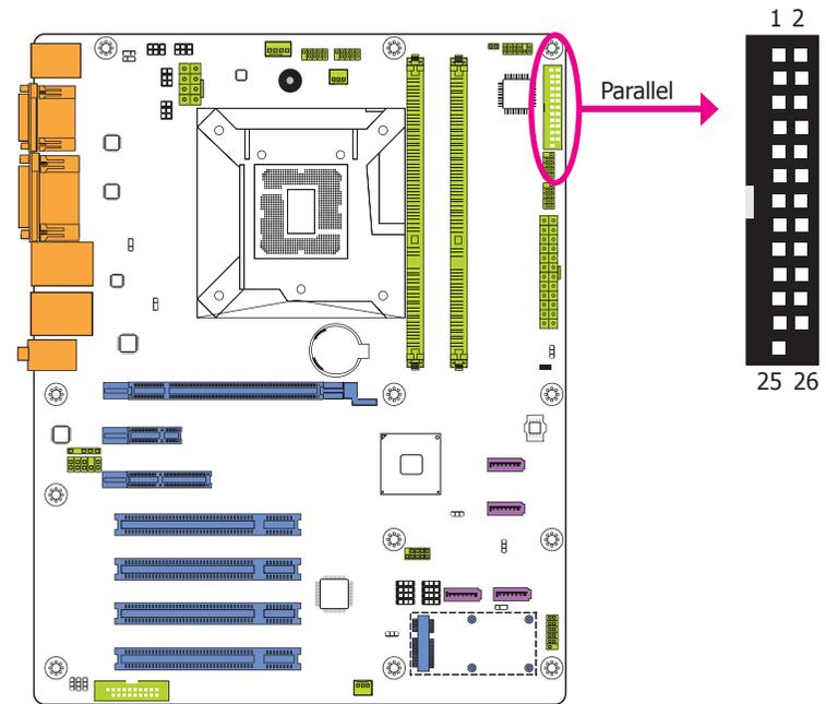
The 25-pin connector is used to connect an external parallel port. The parallel port connects your PC to a parallel printer. It supports SPP, ECP and EPP.
