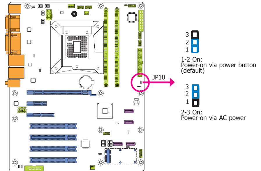
JP10 is used to select the method of powering on the system. If you want the system to power-on whenever AC power comes in, set JP10 pins 2 and 3 to On. If you want to use the power button, set pins 1 and 2 to On.
