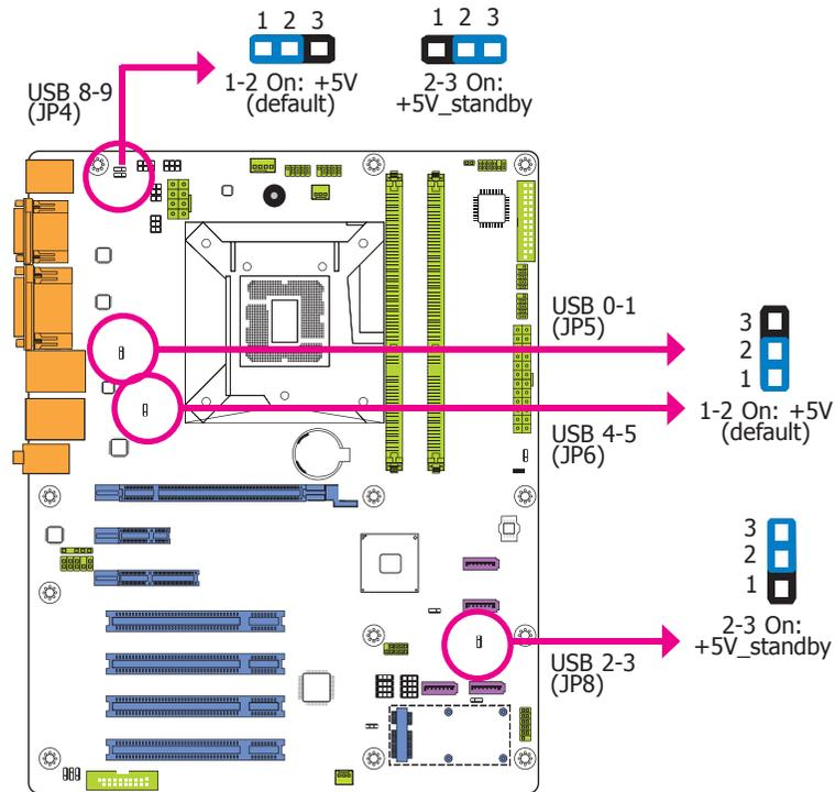
JP4, JP5, JP6 and JP8 are used to select the power of the USB devices. Selecting +5V\_standby will allow you to use a USB device to wake up the system.
