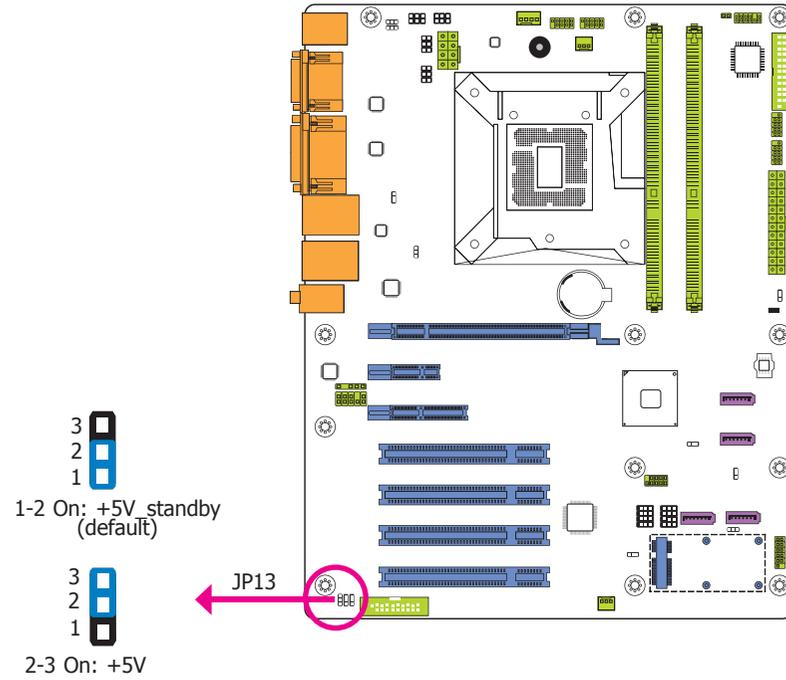
JP13 is used to select the power of DIO (Digital I/O) signal.
