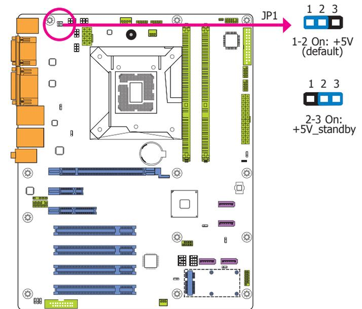
JP1 is used to select the power of the PS/2 keyboard/mouse port. Selecting +5V\_standby will allow you to use the PS/2 keyboard or the PS/2 mouse to wake up the system.
