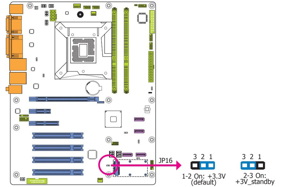
JP16 is used to select the power supplied with the Mini PCIe.
