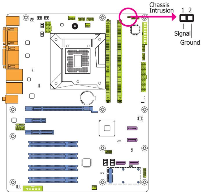
The board supports the chassis intrusion detection function. Connect the chassis intrusion sensor cable from the chassis to this connector. When the system's power is on and a chassis intrusion occurred, an alarm will sound. When the system's power is off and a chassis intrusion occurred, the alarm will sound only when the system restarts.
