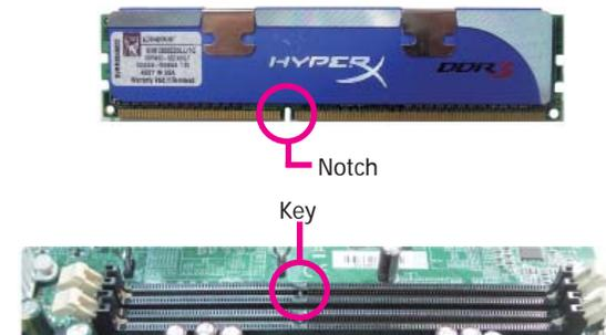
6. Grasping the module by its edges, position the module above the socket with the “notch” in the module aligned with the “key” on the socket. The keying mechanism ensures the module can be plugged into the socket in only one way.
