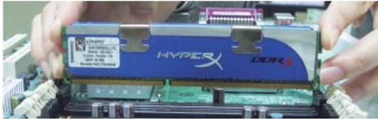
7. Seat the module vertically, pressing it down firmly until it is completely seated in the socket.
