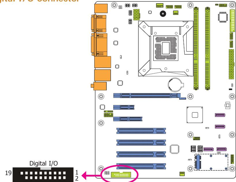
The 8-bit Digital I/O connector provides powering-on function to external devices that are connected to these connectors.
