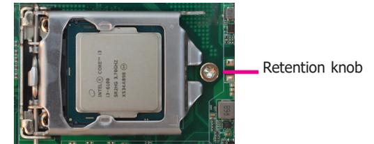
9. Hook the load lever under the retention tab.
