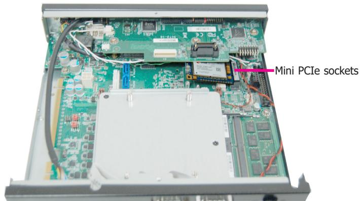
2. Push the Mini PCIe card down and use the provided mounting screw to secure the card on the system board. If antenna cables are used, route them to the antenna holes on the rear panel of the system.
