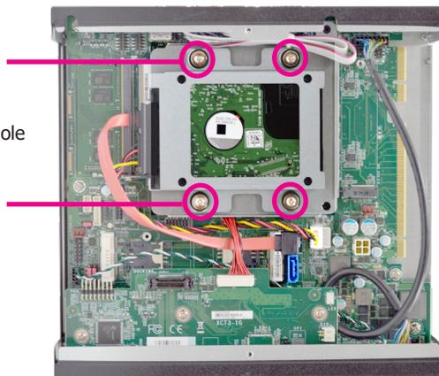
3. Connect the other end of the SATA data and power cable to the SATA data and power connectors on the system board respectively.
