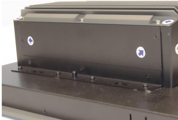
4. Lift the cover upward to open the system.
