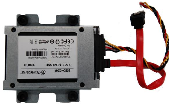
2. Place the SATA drive installed with the HDD bracket in the system. Align the mounting holes on the HDD bracket with the mounting holes on the drive bay and use the provided mounting screws to secure the drive in place.
