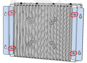
2. Prepare at least four screws (M3, 6 mm) to mount MPT-3000RP on wall .
