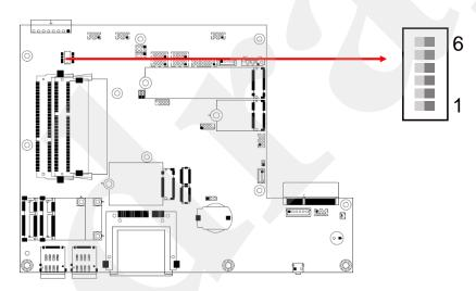
Switch to **ON** to pull high to 5V.
