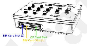
**For micro-SIM card**, insert the card to one of the micro-SIM card slots with the chip down and push the card by using your fingernail or the tip of a pen. Then refer to 2.1.4 *Mini-PCIe* & *M.2 Network Cards Installation* for further installation.
