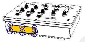
2. The CFast slot and two SIM card slots are indicated below.
