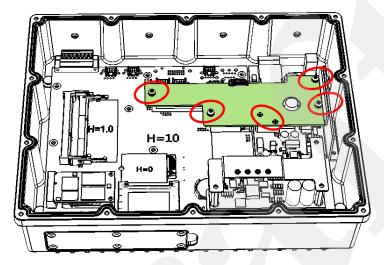
3. Align the key of the new M.2 card to the M.2 interface, and insert the card slantwise.
