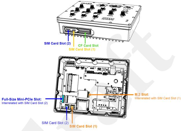
1. Locate the mini-PCIe slot, align the key of the mini-PCIe card to the interface, and insert the card slantwise. (Insert the M.2 network card in the same way.)
