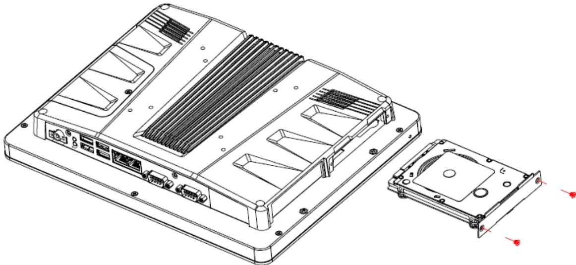
**Step 2.** Remove 4 screws to release the chassis cover, and remove it.
