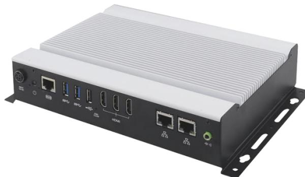
**Warning:** The heatsink temperature becomes high during operation. Be careful not to touch the unit during operation to avoid injury.
