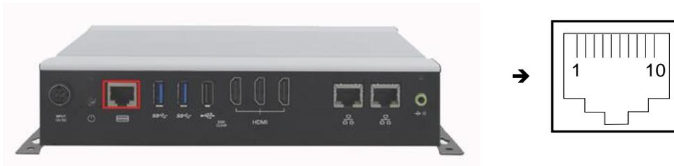
COM1 port is jumper-less and configurable in BIOS.
