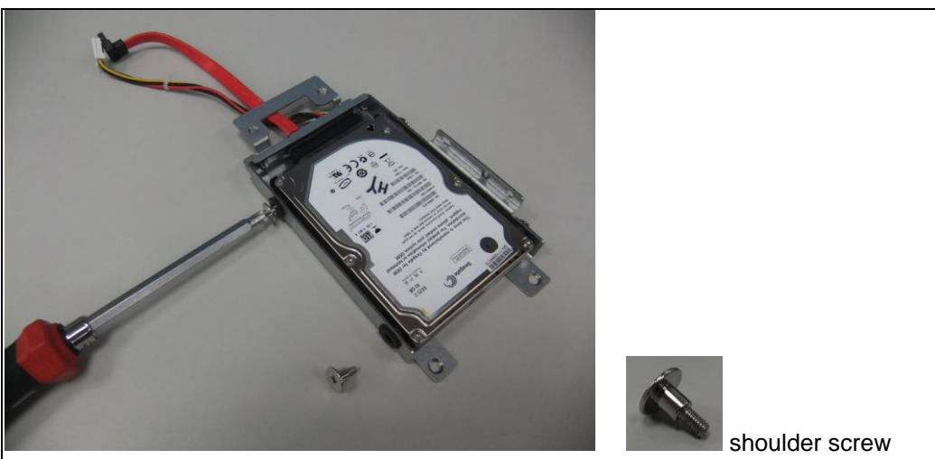
Fig. 6-5 Fasten HDD on bracket with four shoulder screws.
