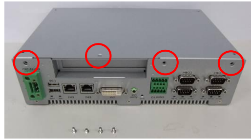
Fig. 4-2 Loosen Four M3 screws on rear & top panel. Top screw is shorter.
