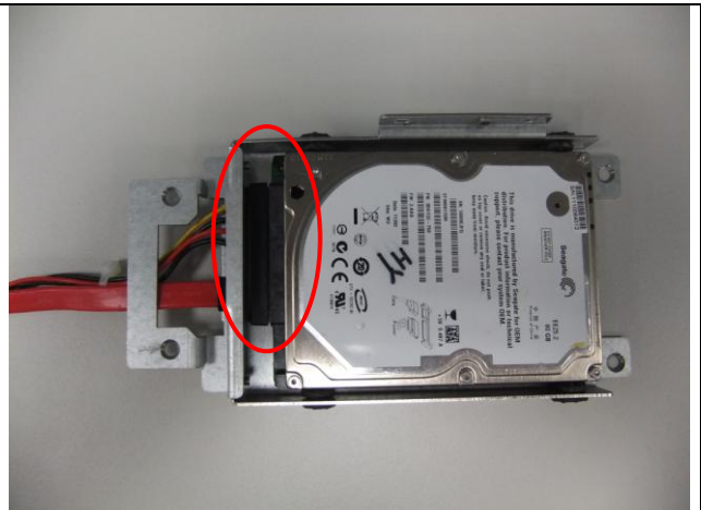
Fig. 6-4 Assemble cable and HDD
