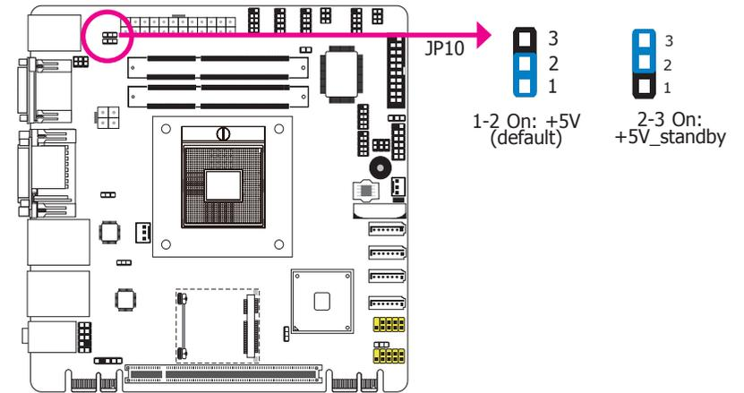
JP10 is used to select the power of the PS/2 keyboard/mouse port. Selecting 5V\_standby will allow you to use the PS/2 keyboard or PS/2 mouse to wake up the system.
