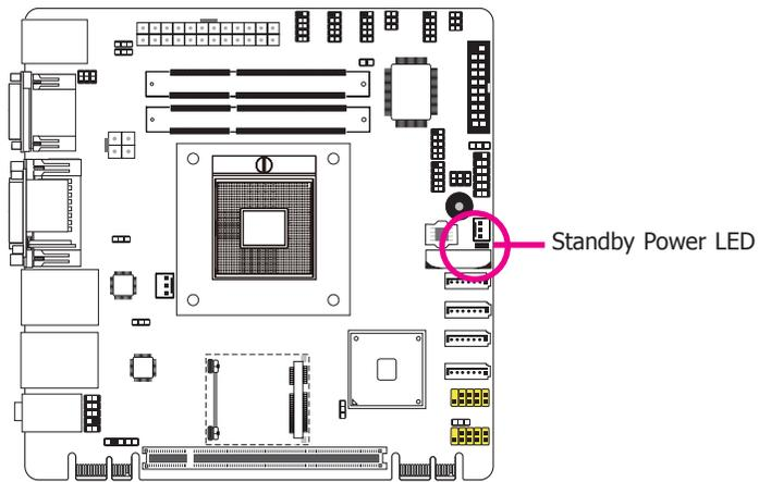
This LED will lit red when the system is in the standby mode. It indicates that there is power on the system board. Power-off the PC and then unplug the power cord prior to installing any devices. Failure to do so will cause severe damage to the motherboard and components.
