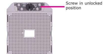
5. Position the CPU above the socket. The gold triangular mark on the CPU must align with pin 1 of the CPU socket.
