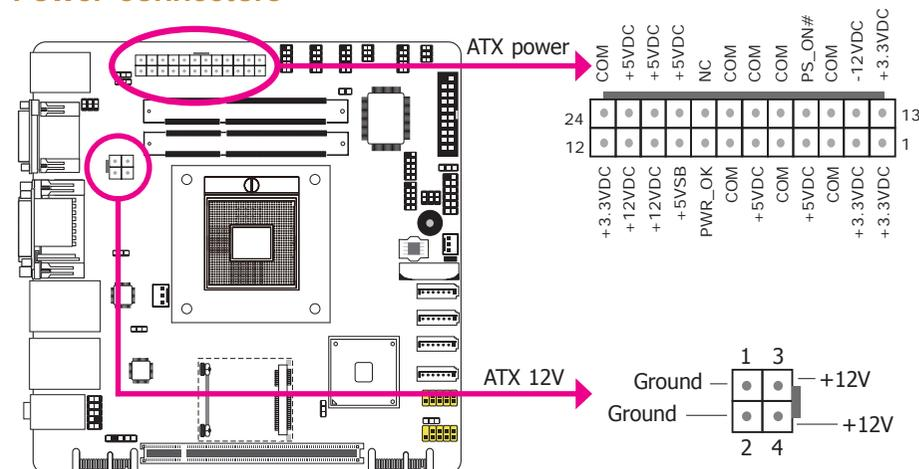
Use a power supply that complies with the ATX12V Power Supply Design Guide Version 1.1. An ATX12V power supply unit has a standard 4-pin ATX main power connector that must be inserted into the 4-pin connector.
