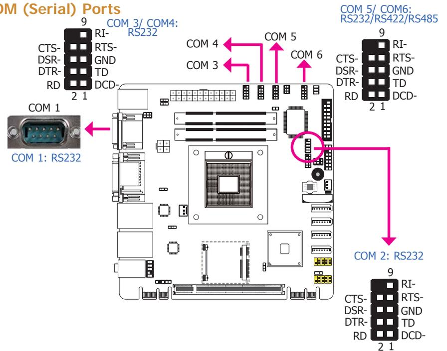
COM 1 to COM 4 are fixed at RS232. The pin function of COM 5 and COM 6 ports will vary according to JP11/JP14's setting. Refer to "COM5/COM6 RS232/RS422/RS485 Select" in this chapter for more information.
