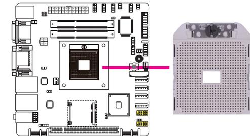
4. Make sure the screw is in its unlock position. If it's not, use a screwdriver to turn the screw to its unlock position.
