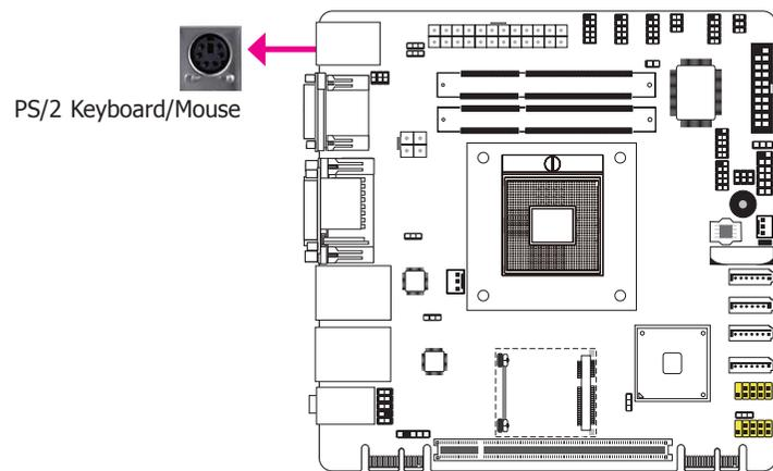
These ports are used to connect a PS/2 mouse and a PS/2 keyboard. The PS/2 mouse port uses IRQ12.
