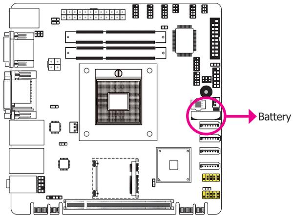
The lithium ion battery powers the real-time clock and CMOS memory. It is an auxiliary source of power when the main power is shut off.
