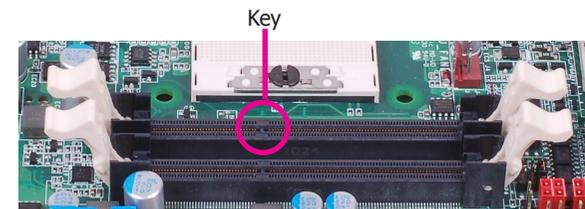
6. Grasping the module by its edges, position the module above the socket with the “notch” in the module aligned with the “key” on the socket. The keying mechanism ensures the module can be plugged into the socket in only one way.
