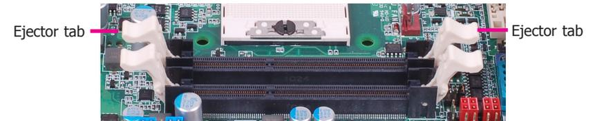
5. Note how the module is keyed to the socket.
