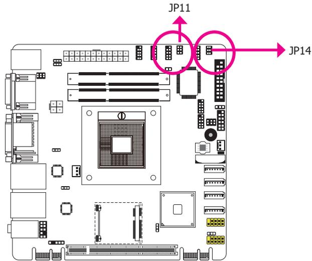
JP11 (for COM5) and JP14 (for COM6) are used to configure the COM ports to RS232, RS422 (Full Duplex) or RS485.
