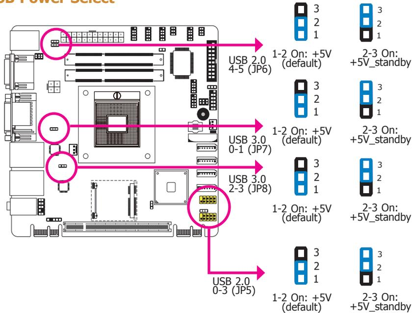
JP5 (for USB2.0 0-3), JP6 (for USB2.0 4-5), JP7 (for USB3.0 0-1) and JP8 (for USB3.0 2-3) are used to select the power of the USB ports. Selecting +5V\_standby will allow you to use a USB device to wake up the system.
