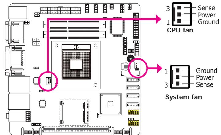
The fan connectors are used to connect cooling fans. The cooling fans will provide adequate airflow throughout the chassis to prevent overheating the CPU and system board components.
