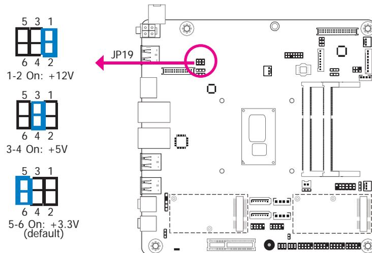
JP19 is used to select the power supplied with the eDP panel.
