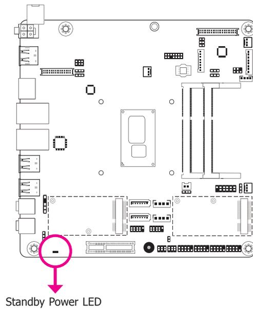
This LED will lit red when the system is in the standby mode. It indicates that there is power on the system board. Power-off the PC and then unplug the power cord prior to installing any devices. Failure to do so will cause severe damage to the motherboard and components.
