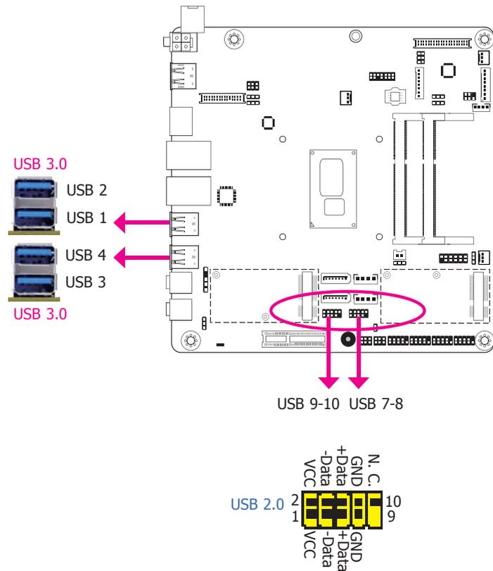
The USB device allows data exchange between your computer and a wide range of simultaneously accessible external Plug and Play peripherals.
