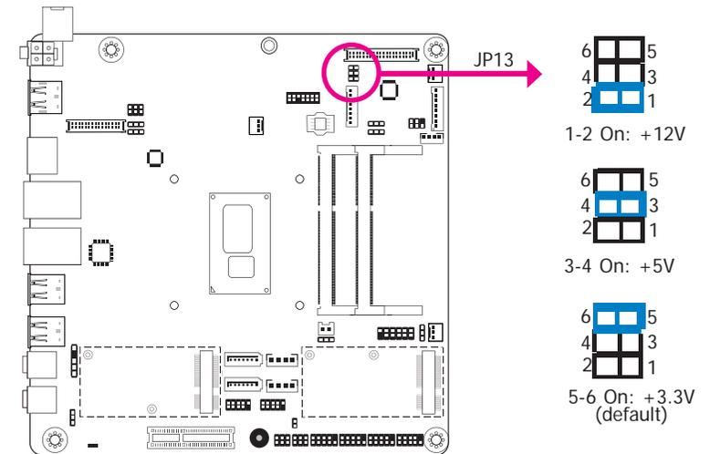
JP13 is used to select the power supplied with the LVDS LCD panel.
