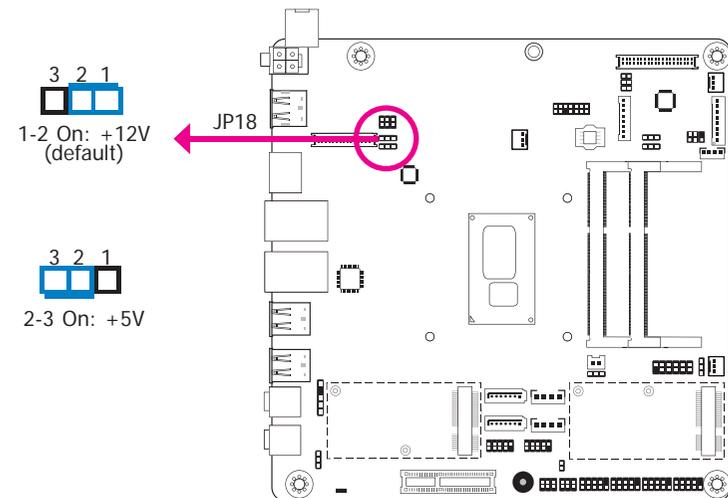
JP18 is used to select the power level of the eDP Inverter power supply.
