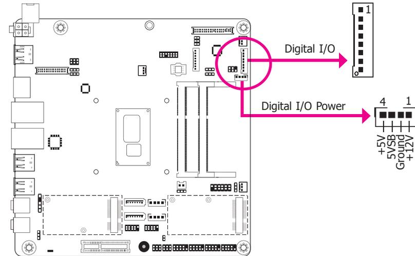
The 8-bit Digital I/O connector provides powering-on function to external devices that are connected to the connector.
