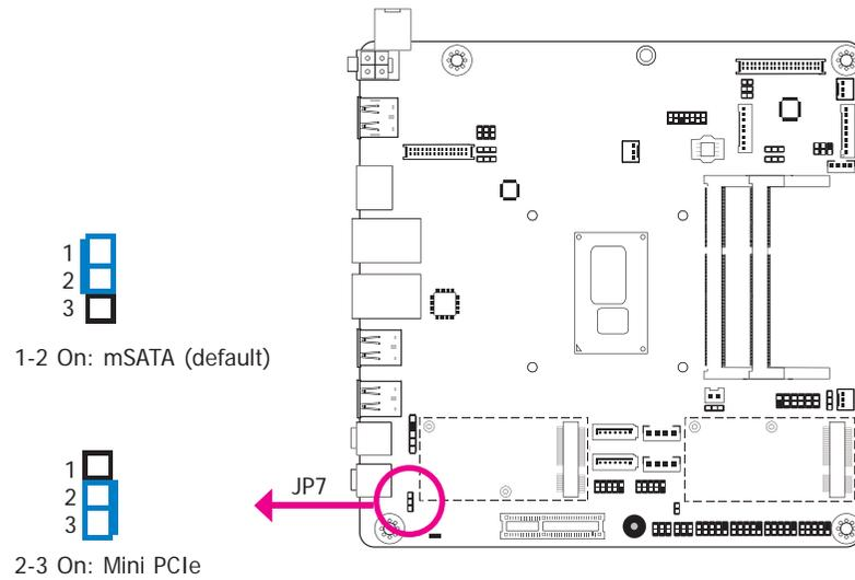
JP7 is used to select the Mini PCIe signal: Mini PCIe or mSATA (default).
