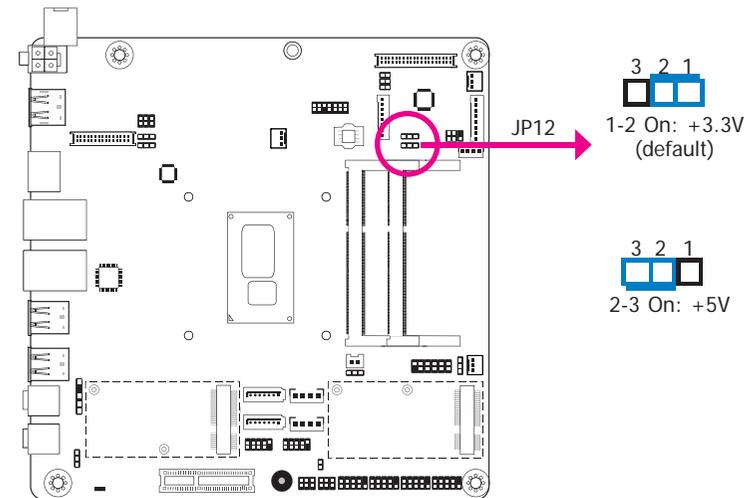
JP12 is used to select the power level of backlight control: +3.3V (default) or +5V.
