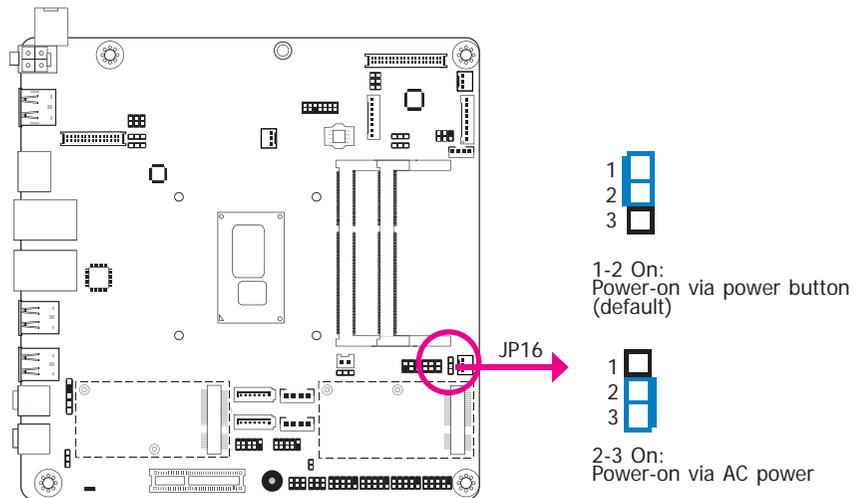
JP16 is used to select the method of powering on the system. If you want the system to power-on whenever AC power comes in, set JP16 pins 2 and 3 to On. If you want to use the power button, set pins 1 and 2 to On.
