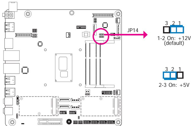
JP14 is used to select the power level of the LCD/Inverter power connector.
