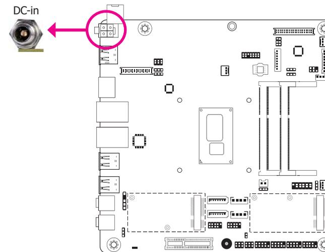
This jack is considered a low power solution. Connect a DC power cord to this jack. Using a voltage more than the recommended range may fail to boot the system or cause damage to the system board.
