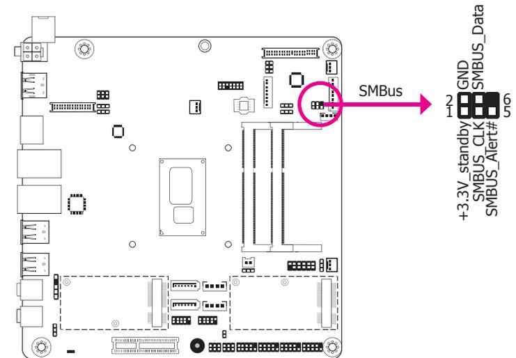
The SMBus (System Management Bus) connector is used to connect SMBus devices. It is a multiple device bus that allows multiple chips to connect to the same bus and enable each one to act as a master by initiating data transfer.
