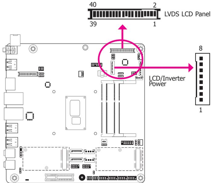
The system board allows you to connect a LCD Display Panel by means of the LVDS LCD panel connector and the LCD/Inverter power connector. These connectors transmit video signals and power from the system board to the LCD Display Panel.
