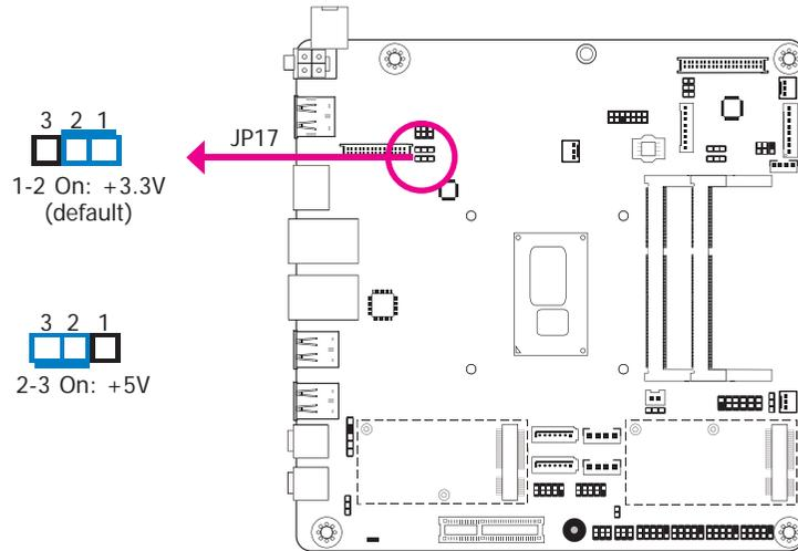
JP17 is used to select the power level of backlight control: +3.3V (default) or +5V.
