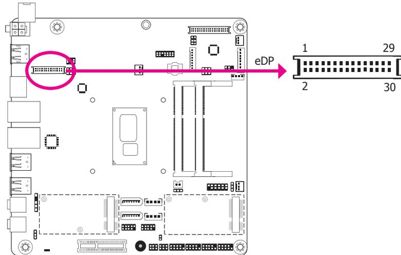
The eDP connector is an embedded displayport which has advanced power-saving features to connect a display device to transmit digital communication of audio and video signals. The table below indicates the pin functions of the eDP connector.
