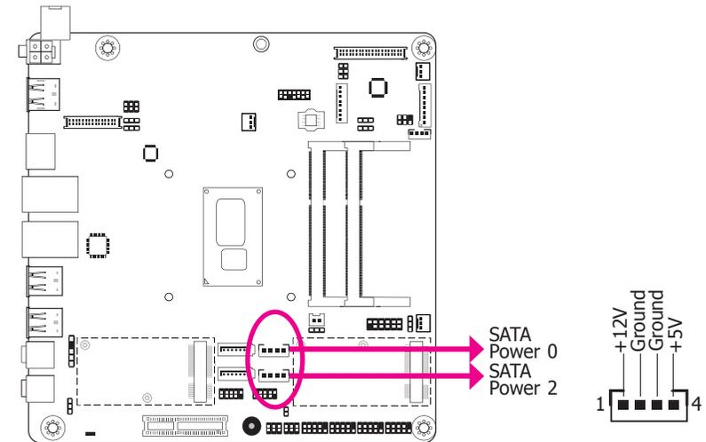
These SATA power connectors supply power to the SATA drive. Connect one end of the provided power cable to the SATA power connector and the other end to your storage device.
