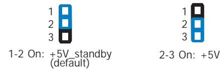
JP3 is used to select the power of DIO (Digital I/O) signal.
