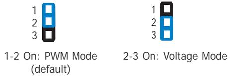
JP6 allows you to select the mode for the lightness control of the LVDS panel.
