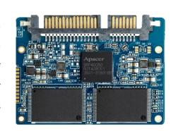
In regard of reliability, the drive comes with various implementations including powerful hardware ECC engine, power saving modes, wear leveling, flash block management, S.M.A.R.T., TRIM, and power failure management.
