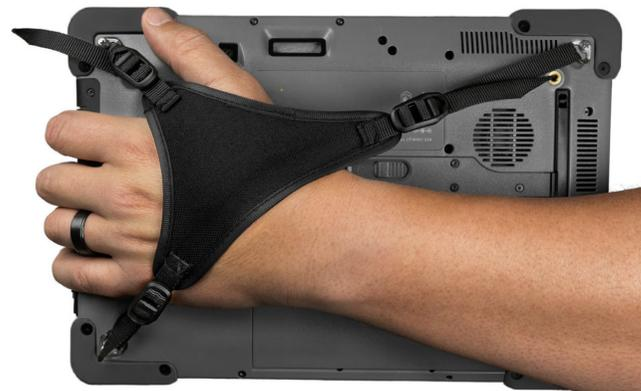
To attach the hand strap, fasten it to three corners as shown in the pictures below.
