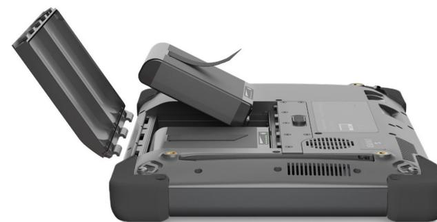
4. Replace the door and press down on it while sliding the latch into the lock position.
