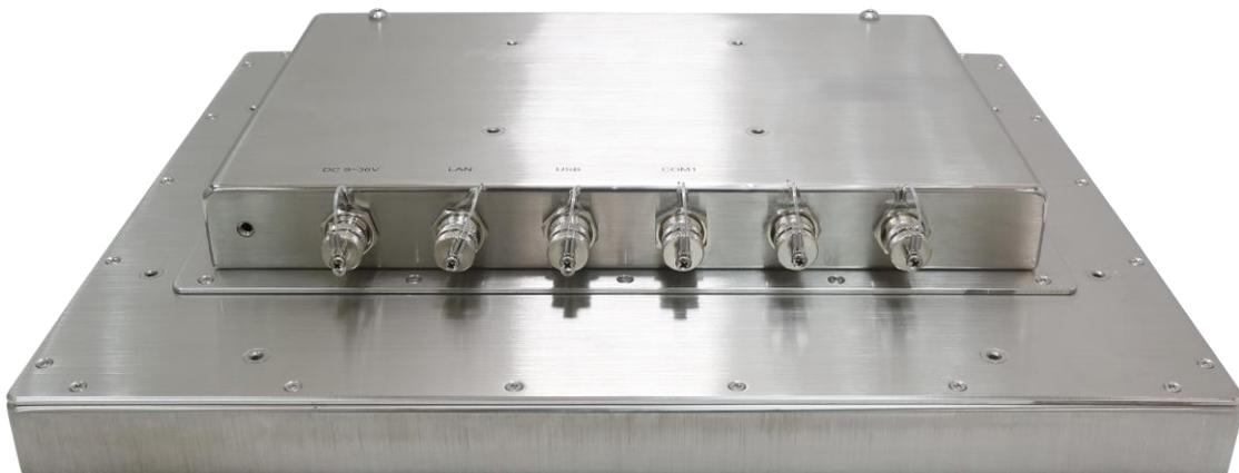
**Figure 1.6: Rear View of AEx-8XXP (H) Series**
