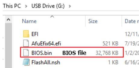
3. Plug the USB drive to the Server and close pin 2-3 of JPFLASHSEC1.
