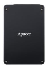
SV25P-25 utilizes 3D NAND for higher capacity up to 960GB and provides more power efficiency than 2D NAND. Regarding reliability, SV25P-25 is built with a powerful SATA controller that supports on-the-module ECC as well as efficient wear leveling scheme and implemented with LDPC (Low Density Parity Check) ECC engine to extend SSD endurance and increase data reliability.
