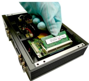
3. Push the memory gently downwards until the slot clips click and lock the memory in place.
