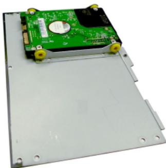
3. Tighten the screws to fix the HDD to the bracket.
