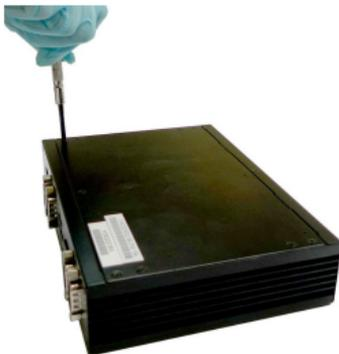
2. Slide the cover carefully sideways and remove it from the system.
