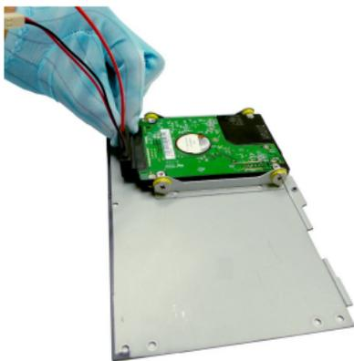
5. Connect the SATA signal & power cable to the motherboard to complete the installation.
