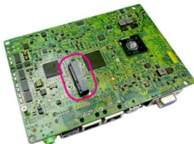
6. Remove the mSATA card screw preinstalled on the motherboard.
