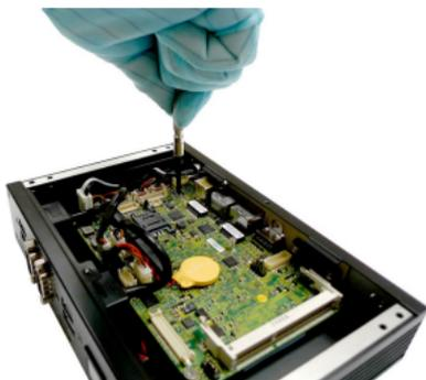
2. Insert the wireless LAN card into the slot at a 45-degree angle.
