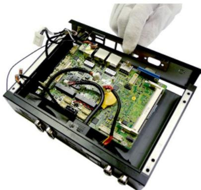
3. Remove the screws that secure the motherboard to the system.
