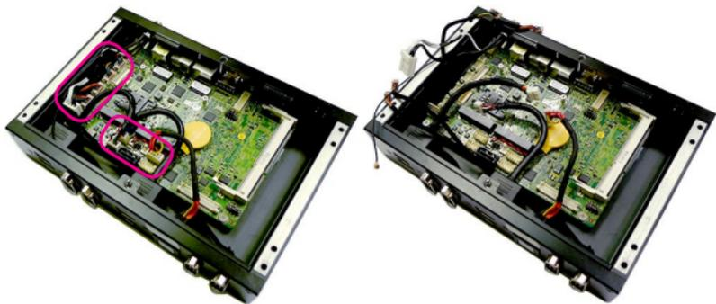
2. Unscrew and remove the system rear panel.
