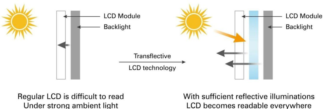
Transflective LCD offers a most convenient and affordable solution for your various outdoor LCD applications such as video systems, kiosk, point-of-sale (POS), etc.
