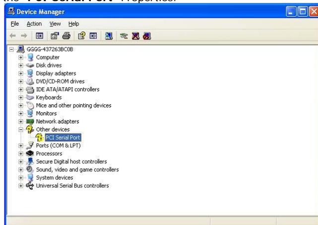
2. In the PCI Serial Port Properties screen, click **Reinstall Driver**.
