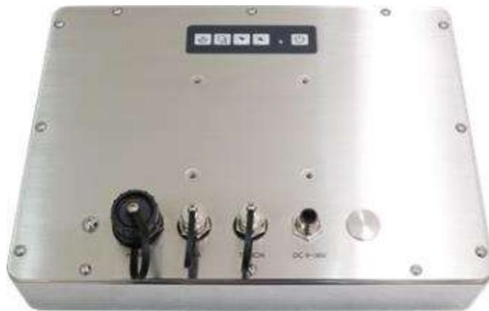
**Figure 1.10: Rear View of ViTAM-110P/R/G/(H)**
