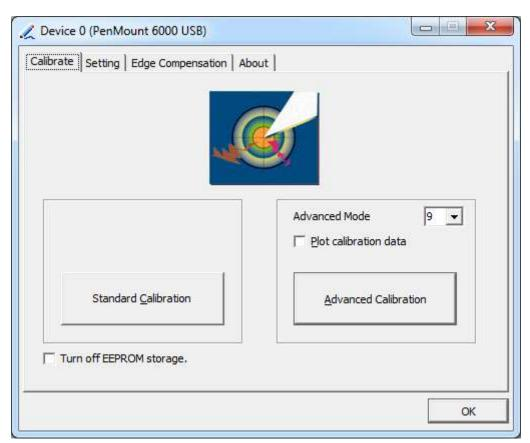
Step 3. Select Device to calibrate, then you can start to do Advanced Calibration.
