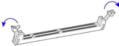
2. Hold the memory module and align the key of the module with that on the memory slot.
