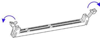
3. Hold the memory module and align the key of the module with that on the memory slot.
