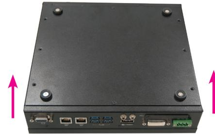
5. The SODIMM sockets, Mini PCIe slot and SATA drive bay are accessible after removing the chassis cover.
