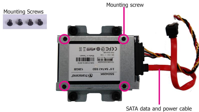
3. Connect the other end of the SATA data and power cable to the SATA data and power connectors on the system board respectively.
