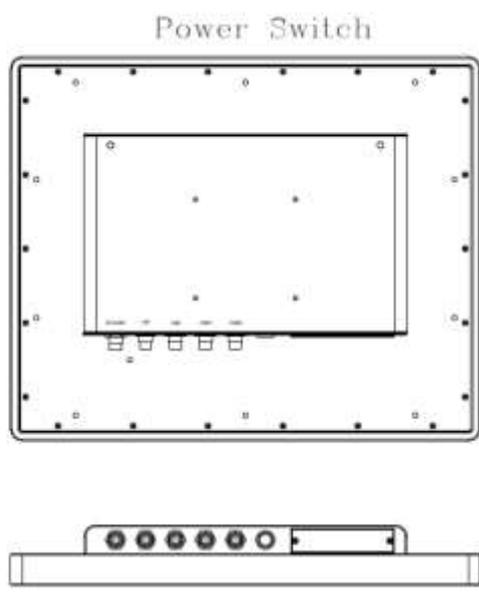
Figure 1.3: Dimensions of APC-3994P/R – Standard & Optional I/O
