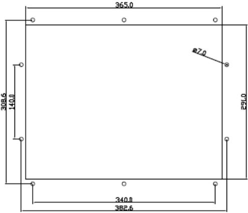
Mounting Hole Size UNIT: mm
