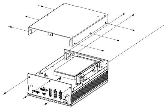
For slots inside the AMI221 & AMI222, you also need to disassemble the intermediate plate by removing the front I/O cover first and then removing 8 screws as shown below.
