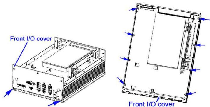
After installation, secure the intermediate plate and the device bottom cover back.
