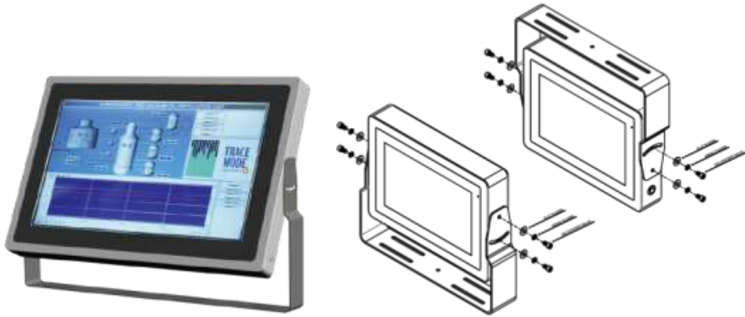
Figure 1.11: Yoke mounting of ViTAM-8XX Series
