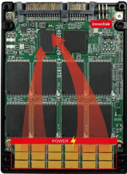
Figure 3: Diagram of 2.5" SATA SSD with iCell
