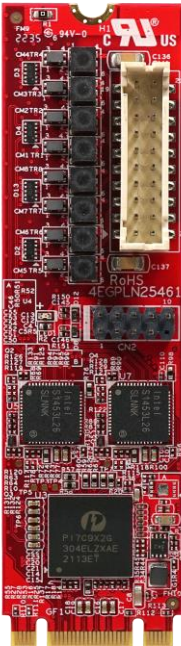
Figure 2: M.2 2280 Board Picture
