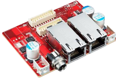
Figure 5: Mounting Hole, DC Jack, Daughter Board Picture (EGPL-G2P1-C3/W3)
