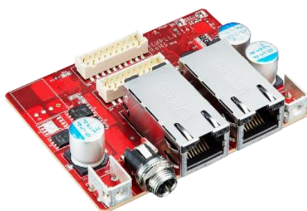
Figure 5: Mounting Hole, DC Jack, Daughter Board Picture (EMPL-G2P1-C3/W3)
