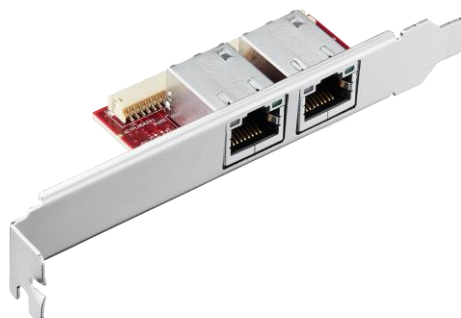
Figure 4: Bracket Daughter Board Picture (EMPL-G2S2-C2/W2)
