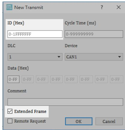
**Extended Frame:** Select to mark this message as an extended message using an extended CAN identifier (ID). The valid value for ID ranges from 00000000 to 1FFFFFFF.
