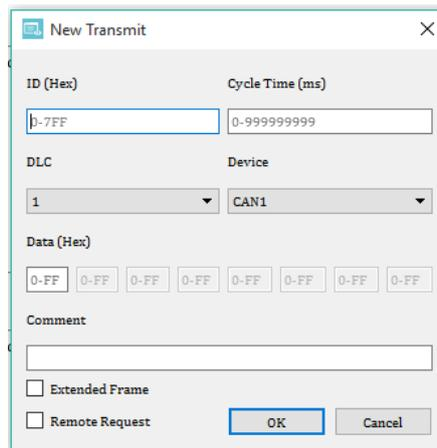
**Device:** Select the CAN port for transmission.
