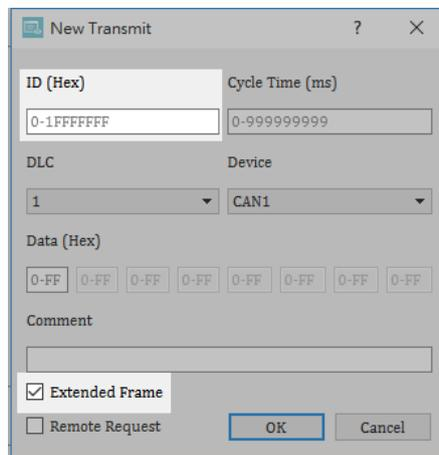
**Remote Request:** Specify that this message being transmitted as a remote request frame with the RTR (remote transmission request) bit equal to 1 (the recessive bit) to differentiate it from a data frame. This type of message contains no data.
