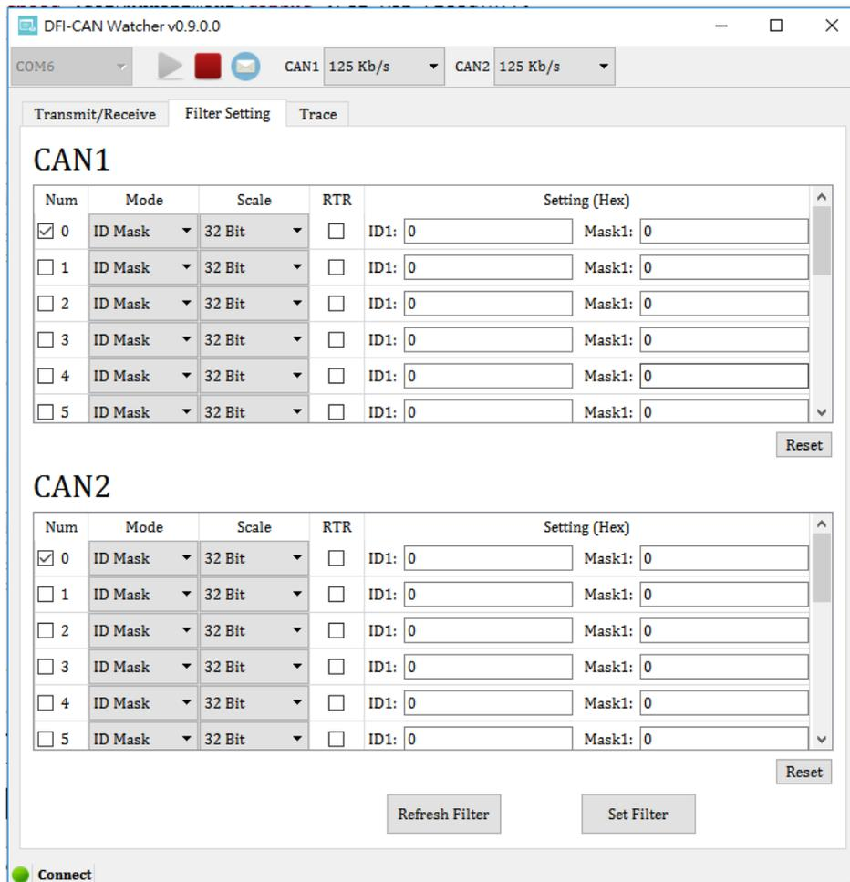
After the application establishes the connection with the DFI CAN module, the configured filters of the DFI CAN module will be loaded first.
