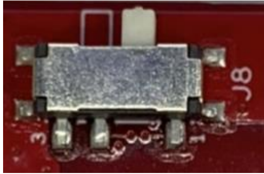
Figure 5: Slide Switch Enable Termination Resistor (J3/J4/J7/J8)
