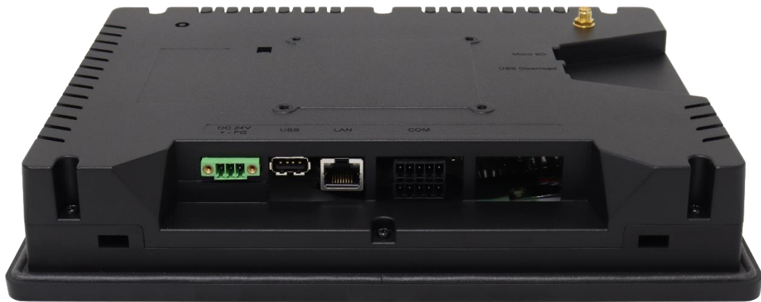
Figure 1.4: Rear View of ARMPAC-6XXB Series
