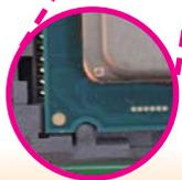
8. Close the load plate then push the load lever down.
